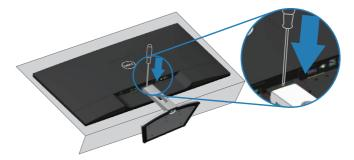
**4.** While pressing on the release button, pull the stand out.
