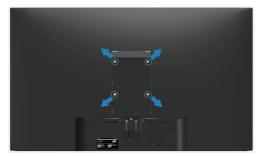
NOTE: For use only with UL-listed wall-mount bracket with minimum weight/load bearing capacity of 30.32 kg.
