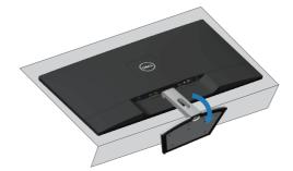
3. Use a long screwdriver to press on the release button.
