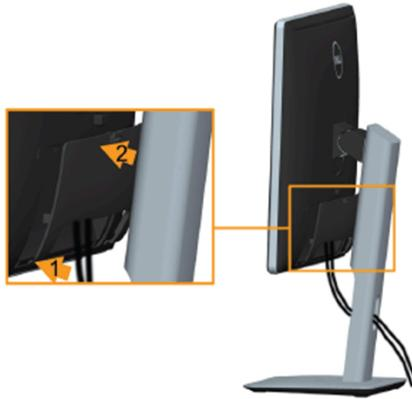
1. Fit the two tabs on the bottom part of the Cable Cover to the groove on the back of the monitor.
