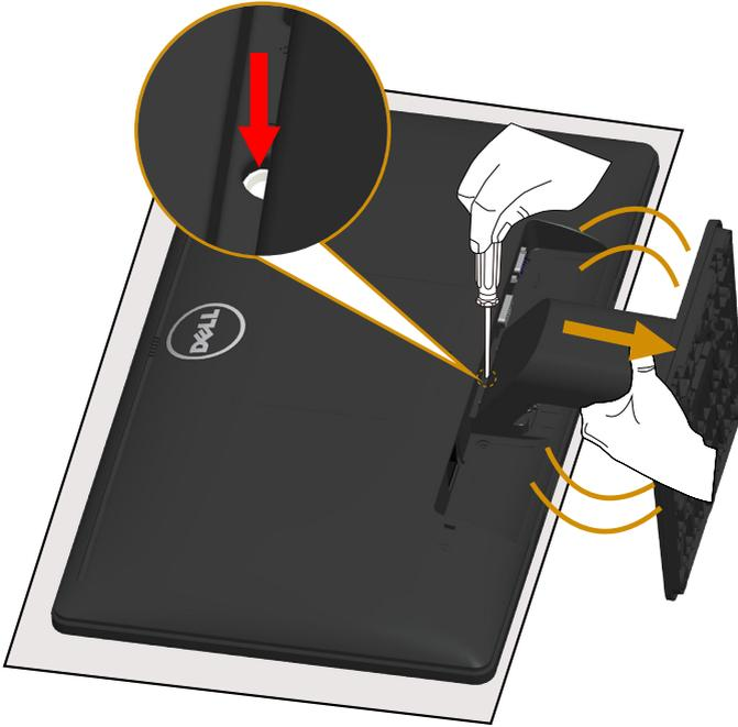
After placing the monitor panel on a soft cloth or cushion, complete the following steps to remove the stand:
