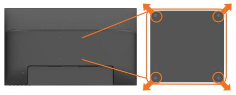
**NOTE:** Use M4 x 10 mm screws to connect the monitor to the wall-mounting kit.
