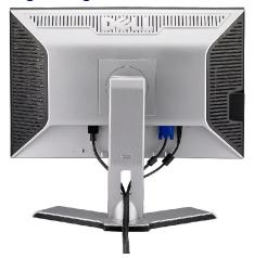
After attaching all the necessary cables to your monitor and computer, (See <u>Connecting Your Monitor</u> for cable attachment,) use the cable management slot to organize all cables as shown above.
