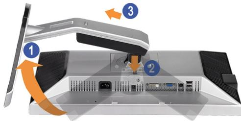
1. Rotate the stand to allow access to the stand release button.
