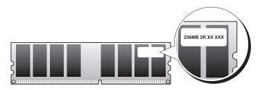
**NOTE:** Always install DDR2 memory modules in the order indicated on the system board.
