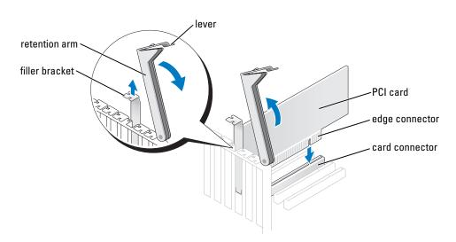
**3** If you are upgrading to a dual-graphics configuration, remove the filler bracket to create a card-slot opening.
