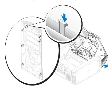
Close the computer cover halfway and pull the front panel away from the computer.
