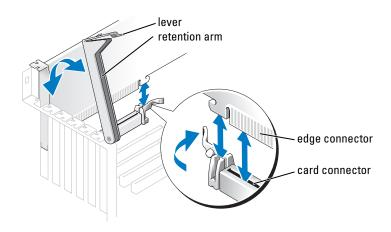
**5** Pull the securing tab (if present), grasp the card by its top corners, and ease it out of its connector.
