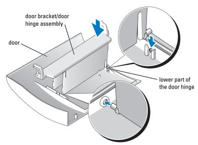
**3** Attach the drive door to the computer, starting with the bottom bracket hinge.
