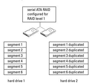
If a drive failure occurs, subsequent read and write operations are directed to the surviving drive. A replacement drive can then be rebuilt using the data from the surviving drive. Also, because data is duplicated on both drives, a RAID level 1 configuration using two 120-GB hard drives collectively has a maximum of 120 GB on which to store data.
