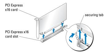
NOTICE: Ensure that you release the securing tab to seat the card. If the card is not installed correctly, you may damage the system board.
