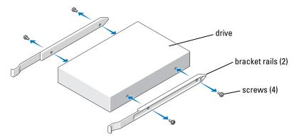
**3** Gently slide the drive into place until the tabs securely click into position.
