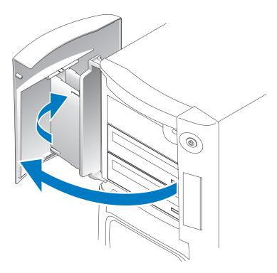
**2** Unsnap the top bracket hinge and pull the top of the drive door outward, away from the computer.
