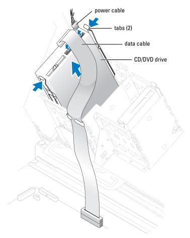
Press inward on the two tabs on the sides of the drive, and then slide the drive upward and remove it from the drive bay.
