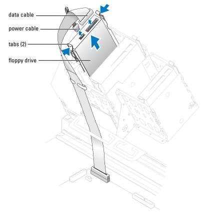
**4** Press inward on the two tabs on the sides of the drive, slide the drive upward, and remove it from the floppy-drive bay.
