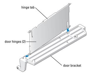
**2** Attach the door bracket/door hinge assembly to the door, starting with the lower part of each door hinge.
