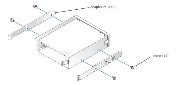
**6** Slide the adapter into the 5.25-inch drive bay until the tabs on the rails securely click into position.
