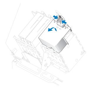
**3** Disconnect the power and hard-drive cables from the drive and from the system board.
