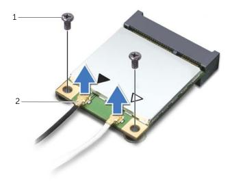
1 screws (2) 2 antenna cables (2) 3 Slide and remove the wireless mini-card out of the wireless mini-card connector.
