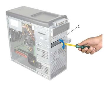
1 break-away metal plate **3** Gently slide the third hard-drive into the hard-drive bay through the front of the computer.
