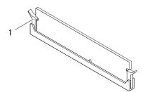
1 securing clip (snapped in position)
