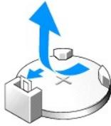
5. Remove the battery by prying it out of its socket with your fingers.
