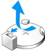
5. Remove the battery by prying it out of its socket with your fingers.
