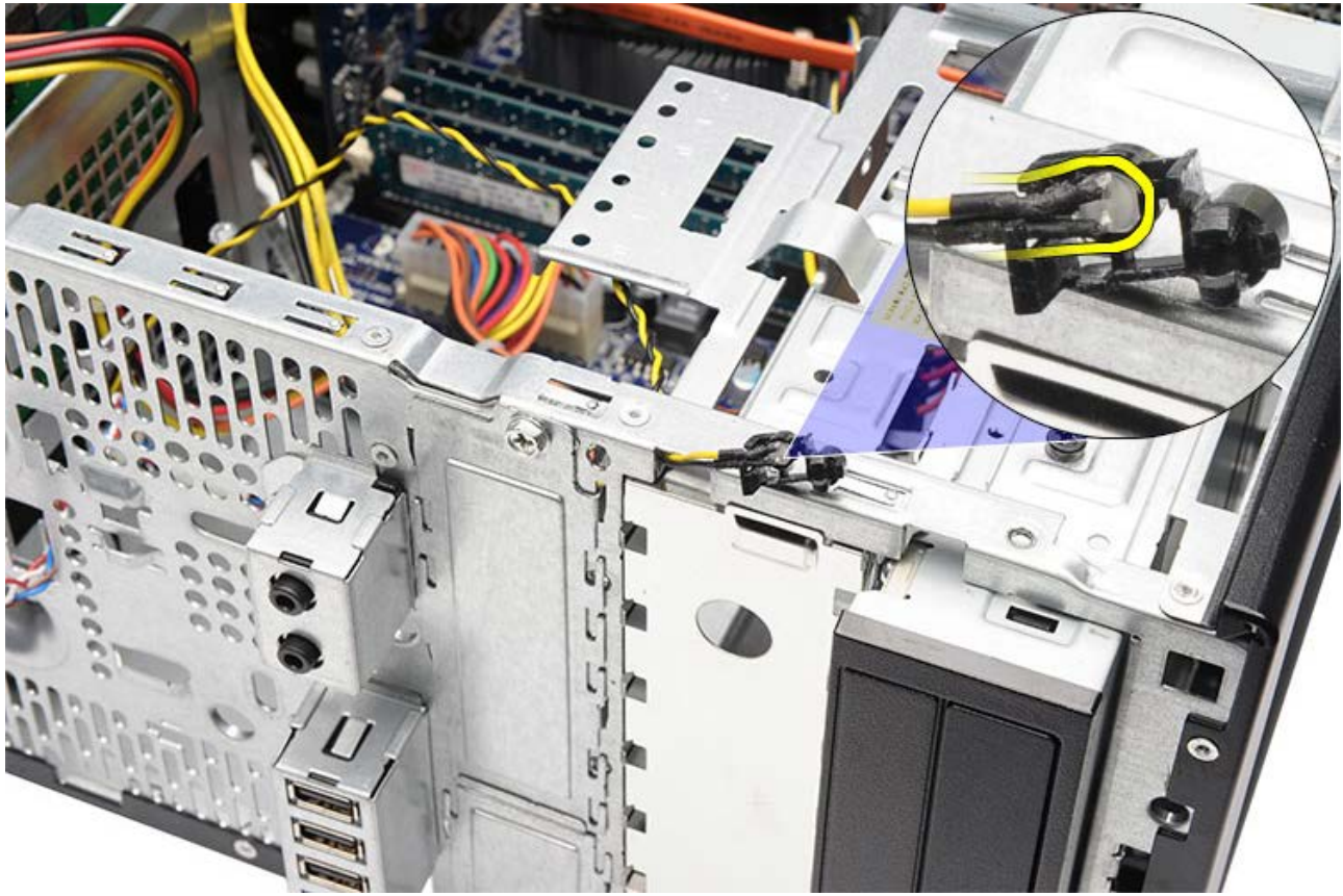
7. Disconnect the power button cable from the system board.
