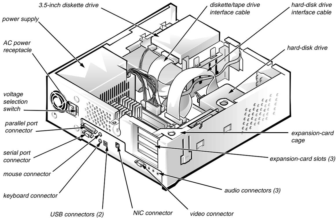
**Figure 1-3. Internal View of the Low-Profile Computer**
