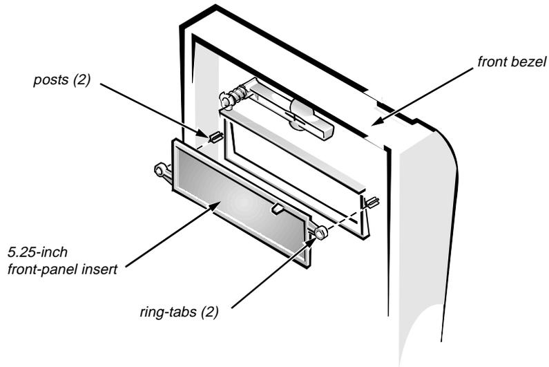
**Figure 6-4. 5.25-Inch Front-Panel Insert Removal**
