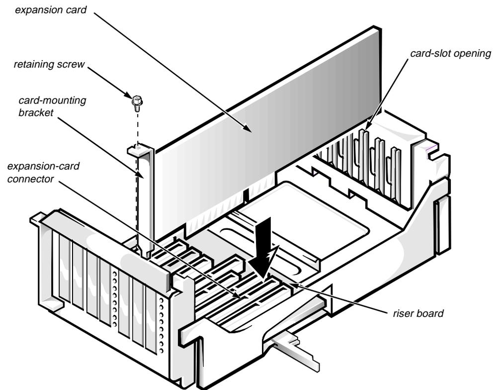
**Figure 6-17. Expansion-Card Removal**
