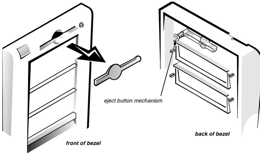
**Figure 6-5. 3.5-Inch Front-Panel Insert Removal**
