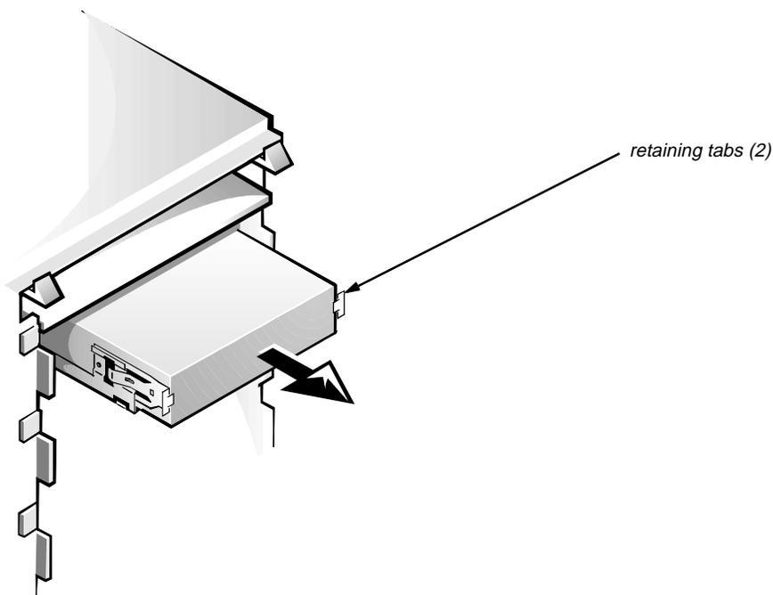
**Figure 6-10. 5.25-Inch Drive Assembly Removal**
