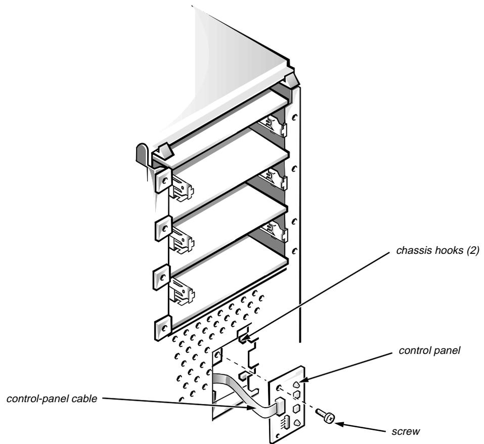
**Figure 6-6. Control-Panel Removal**
