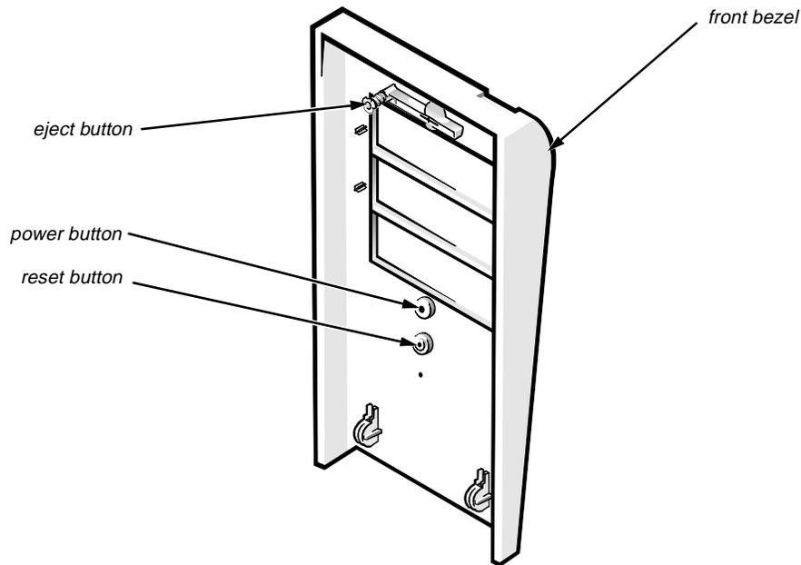
**Figure 6-3. Eject, Power, and Reset Button Removal**
