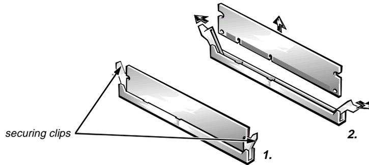
**Figure 6-19. DIMM Removal**
