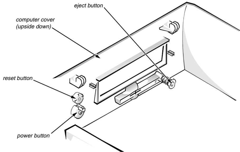
**Figure 4-2. Eject, Power, and Reset Button Removal**
