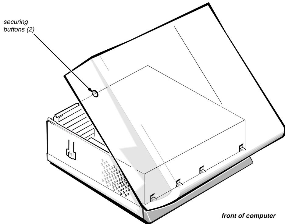
**Figure 5-2. Computer Cover Removal**
