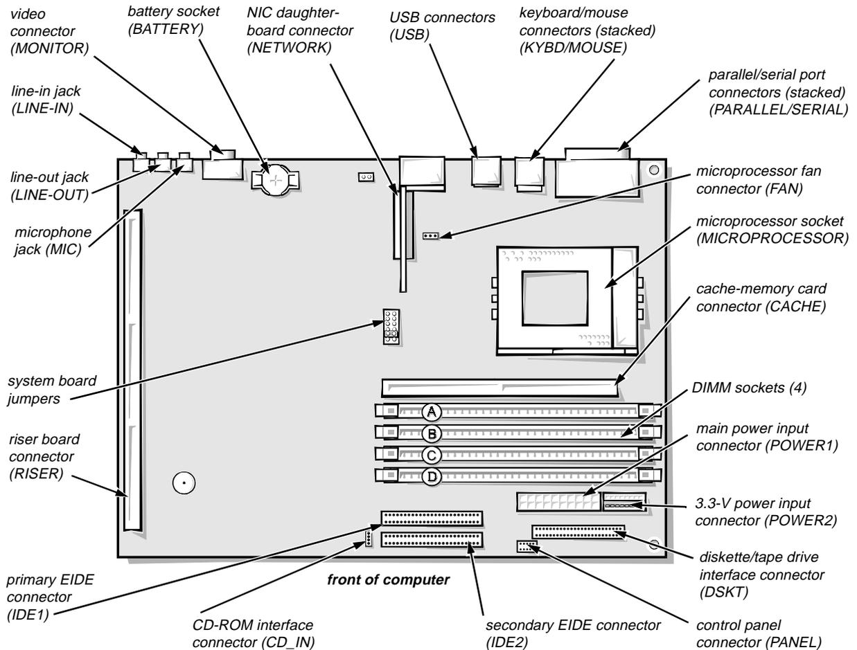
**Figure 1-19. System Board Components**
