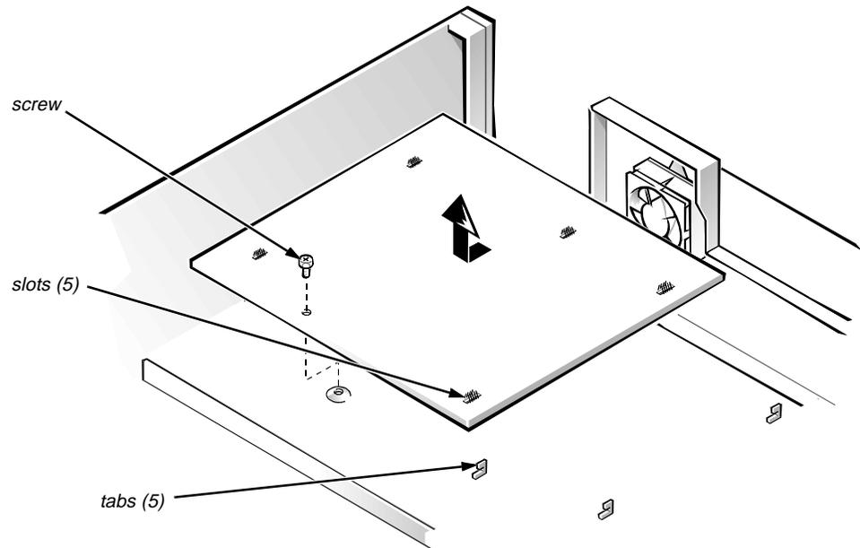
**Figure 6-26. System Board Removal**
