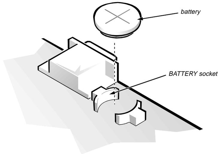
**Figure 5-23. System Battery Removal**
