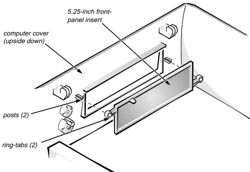
**Figure 4-3. Front-Panel Insert Removal**
