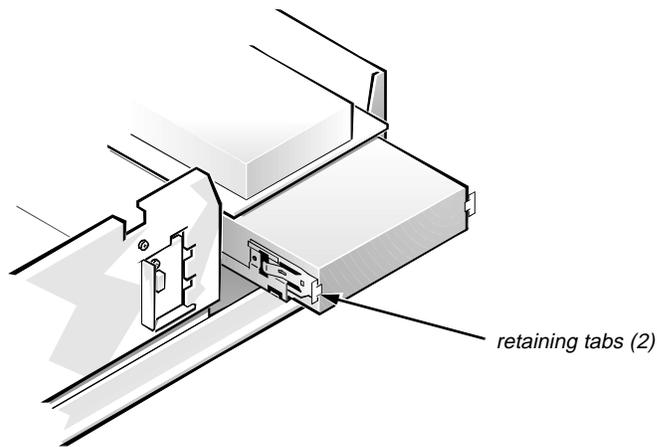
**Figure 5-8. 5.25-Inch Drive Assembly Removal**
