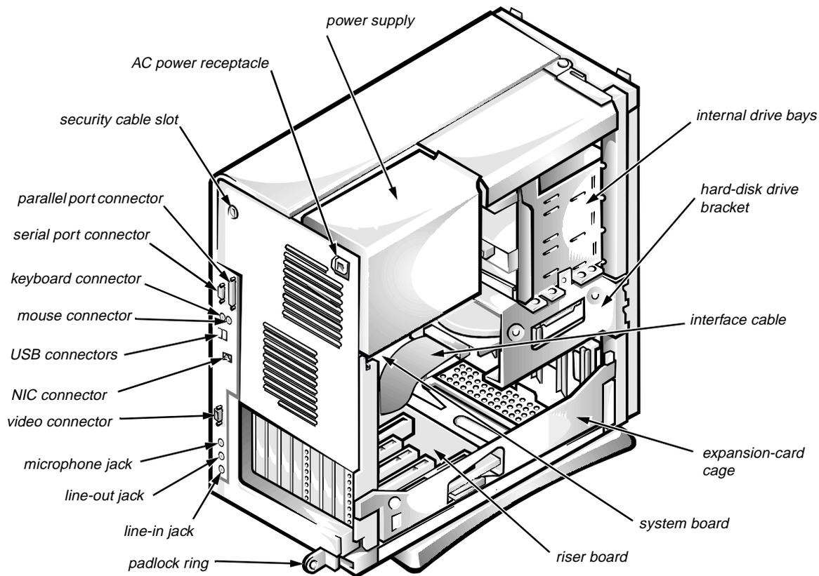
**Figure 1-5. Internal View of the Mini Tower Computer**
