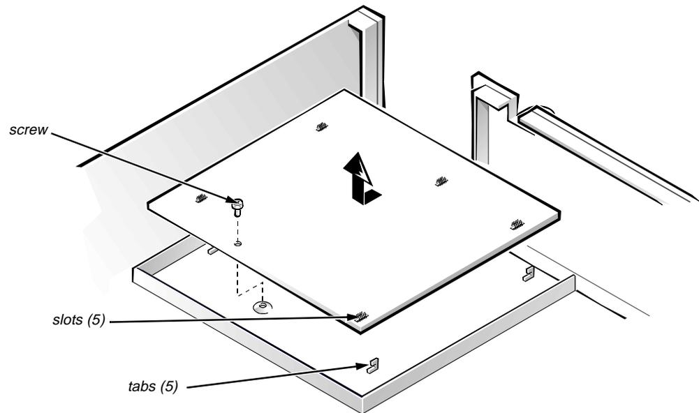
**Figure 4-21. System Board Removal**
