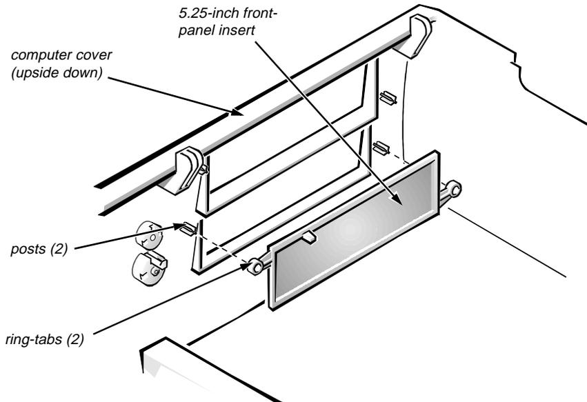
**Figure 5-4. Front-Panel Insert Removal**
