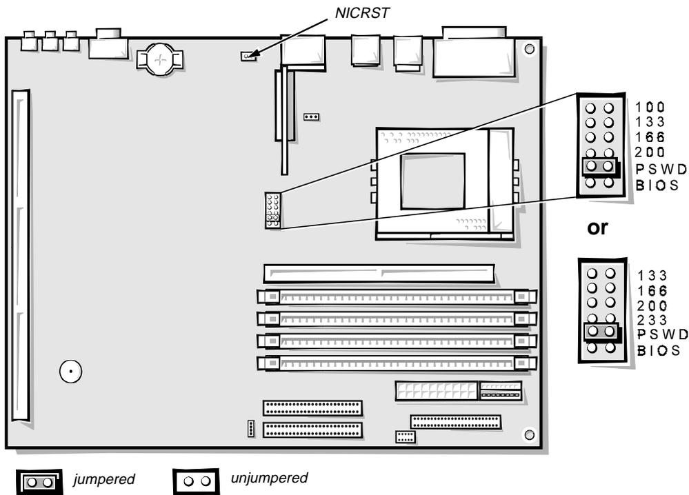
**Figure 1-20. System Board Jumpers**
