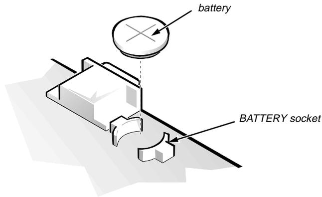
**Figure 4-20. System Battery Removal**
