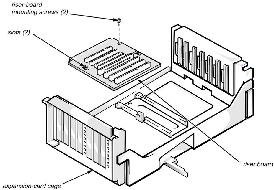
**Figure 6-18. Riser Board Removal**
