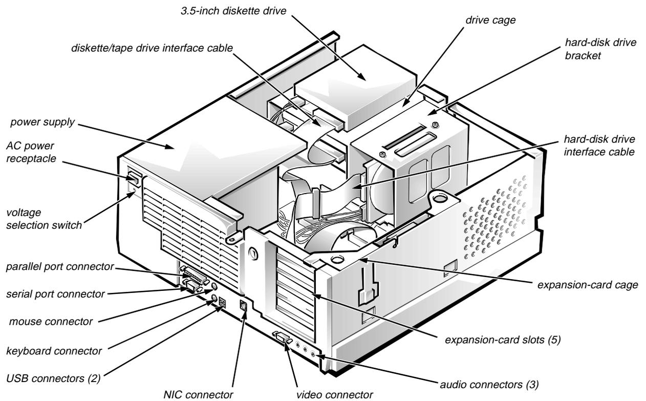
**Figure 1-4. Internal View of the Midsize Computer**
