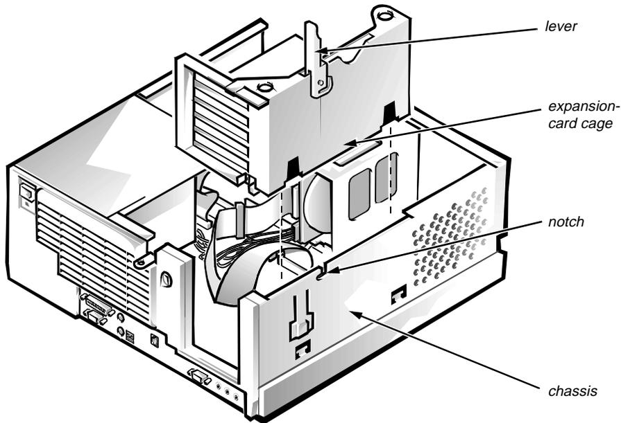
**Figure 5-14. Expansion-Card Cage Removal**
