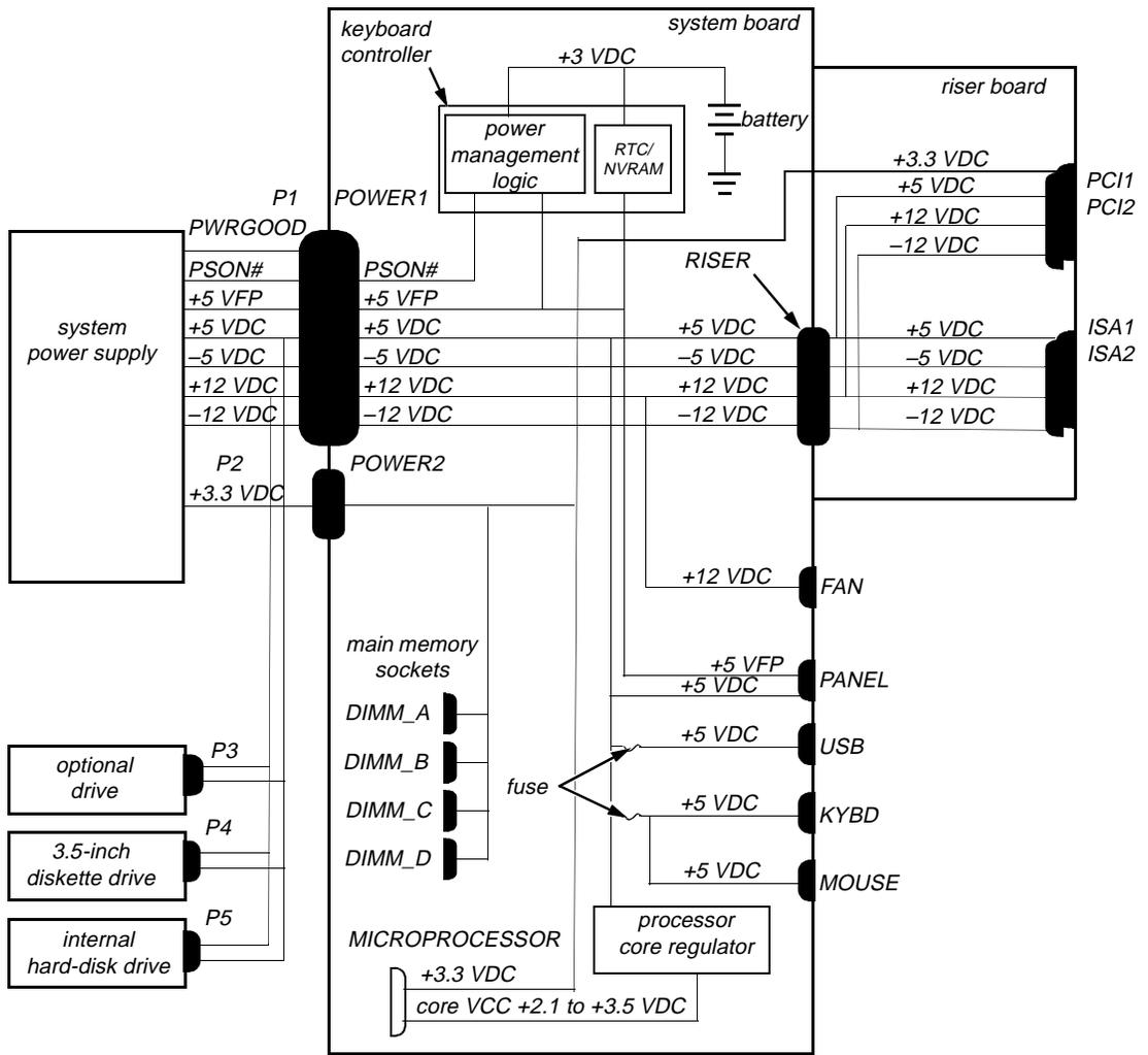
**Figure 1-15. DC Power Distribution for the Low-Profile Computers**
