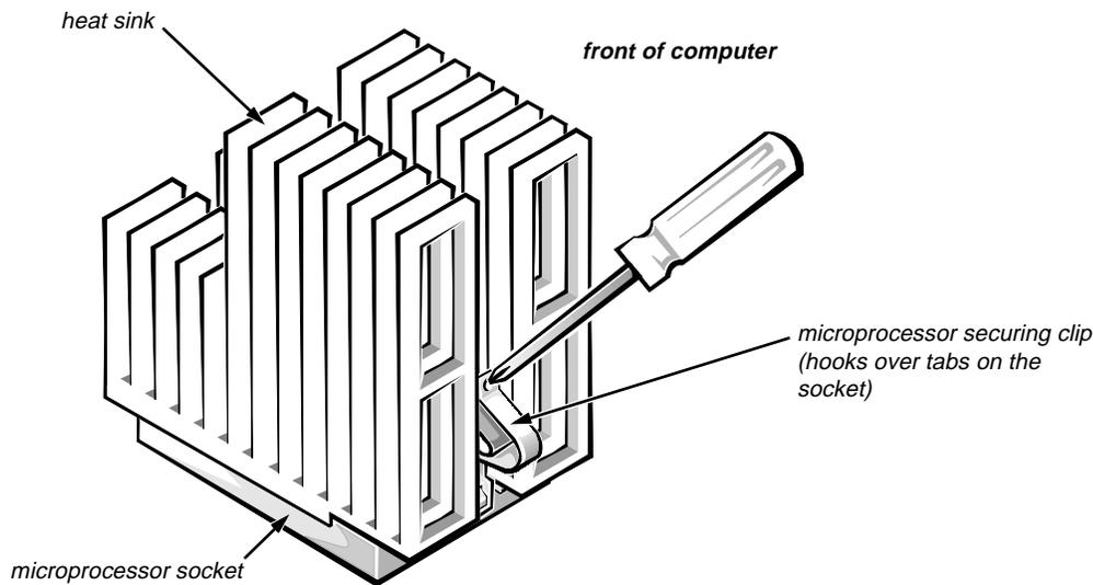
**Figure 4-18. Microprocessor Securing-Clip Removal**
