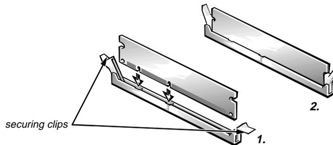
***Figure 5-18. DIMM Installation***
