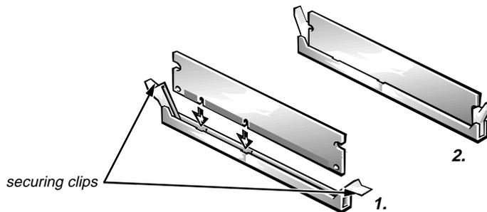
**Figure 6-20. DIMM Installation**
