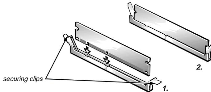
**Figure 4-15. DIMM Installation**
