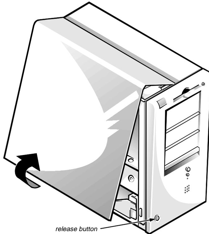
**Figure 6-1. Computer Cover Removal**
