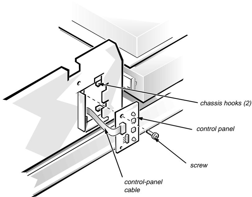
**Figure 5-5. Control-Panel Removal**
