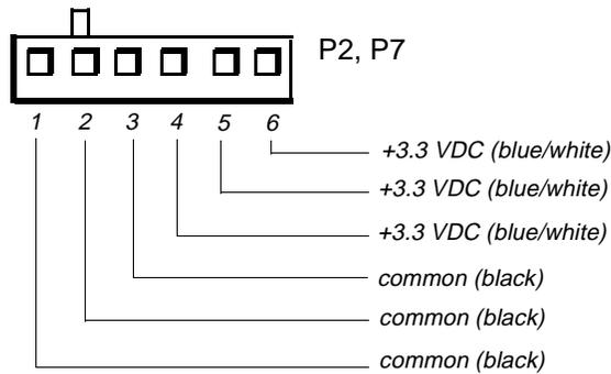
**Figure 1-13. DC Power Connectors P2 (Low-Profile) and P7**
