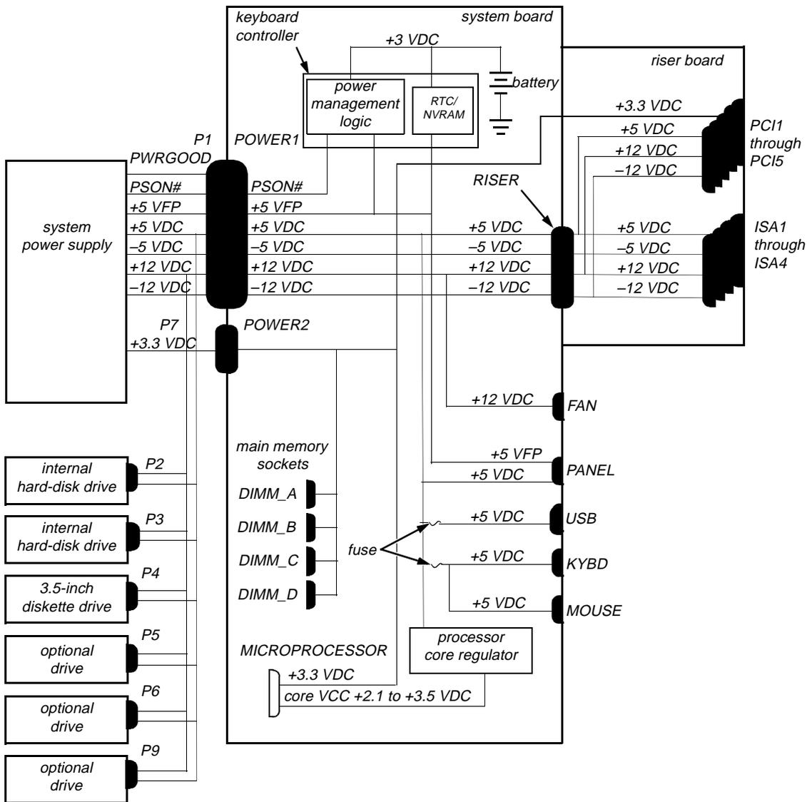
**Figure 1-18. DC Power Distribution for the Mini Tower Computers**
