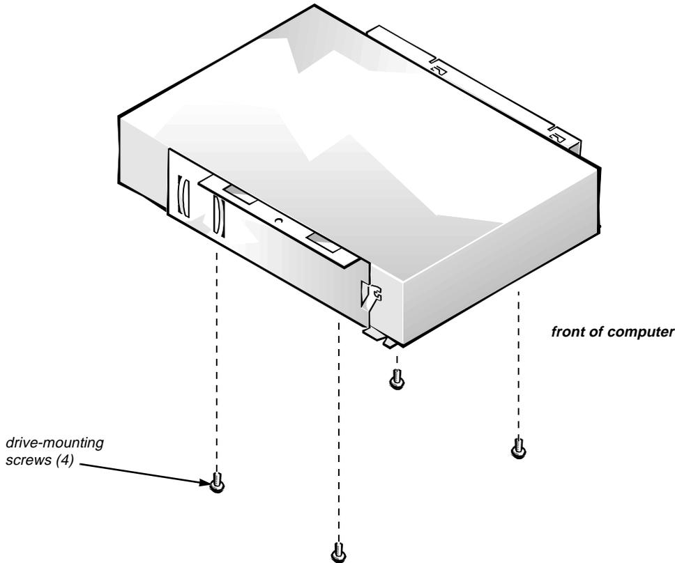
**Figure 4-7. 5.25-Inch Drive Assembly Removal**
