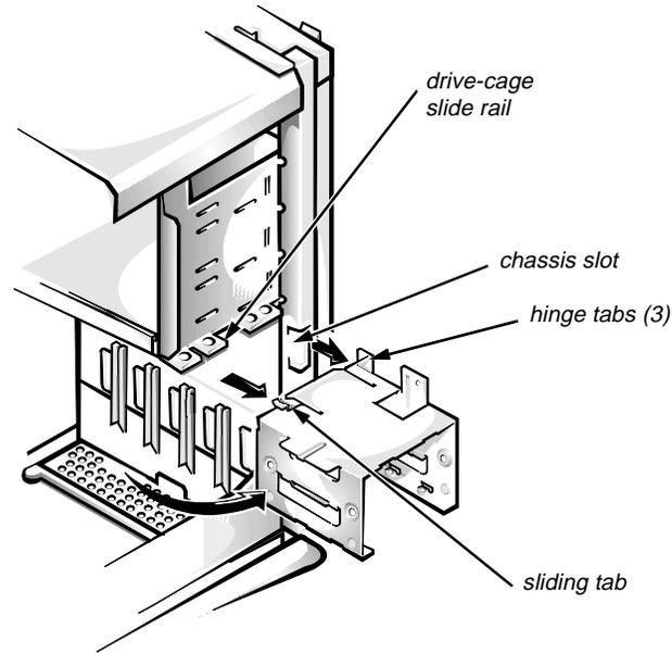
**Figure 6-12. Hard-Disk Drive Bracket Removal**
