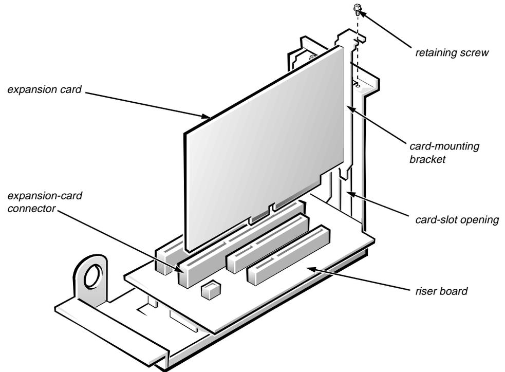
**Figure 4-12. Expansion-Card Removal**
