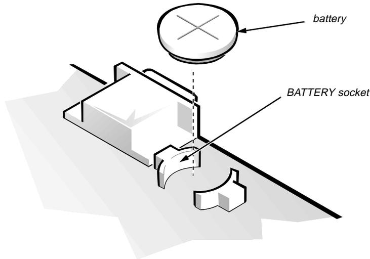
**Figure 6-25. System Battery Removal**
