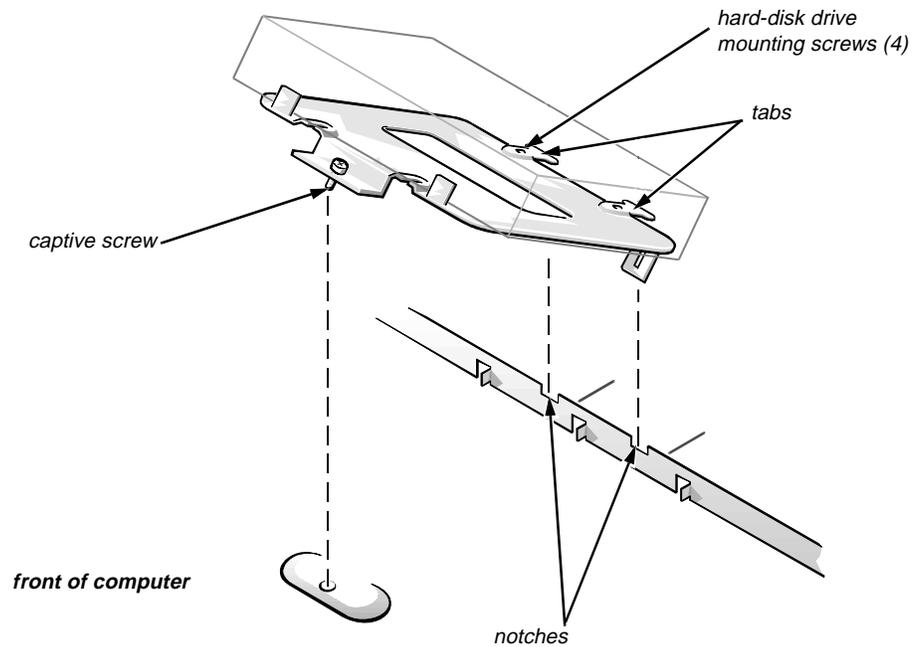
**Figure 4-8. Hard-Disk Drive Assembly Removal**
