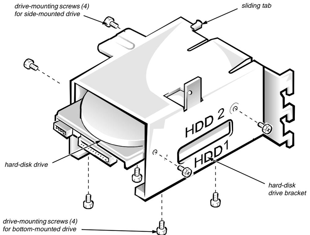
**Figure 6-13. Hard-Disk Drive Removal**
