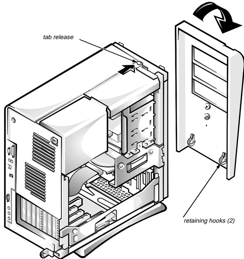
**Figure 6-2. Front Bezel Removal**
