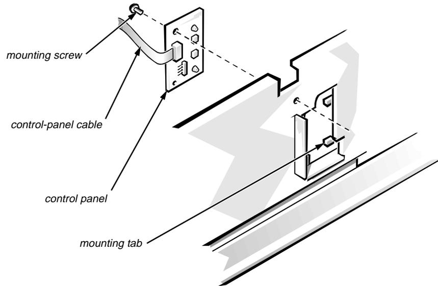
**Figure 4-4. Control-Panel Removal**
