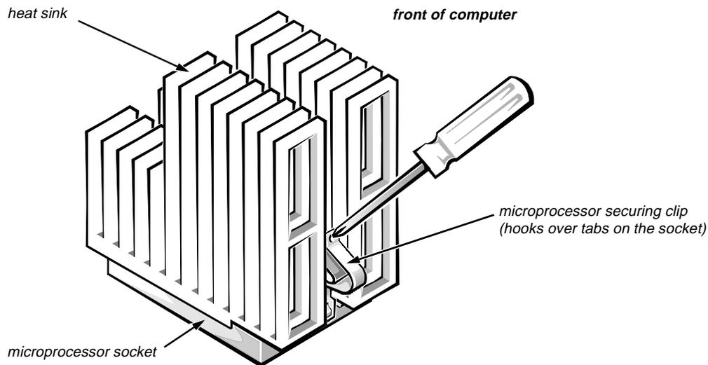
**Figure 5-21. Microprocessor Securing-Clip Removal**
