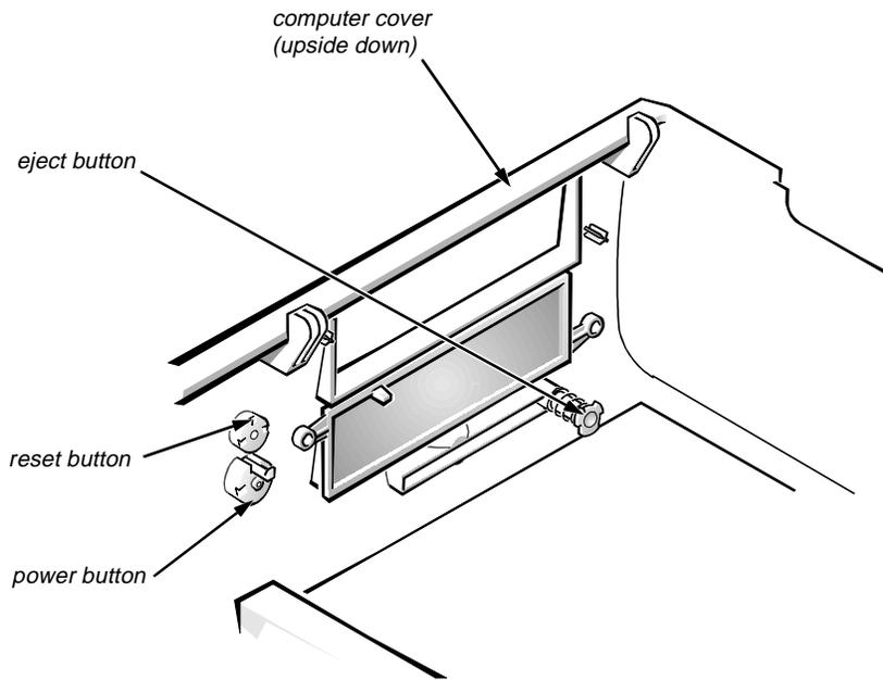
**Figure 5-3. Eject, Power, and Reset Button Removal**
