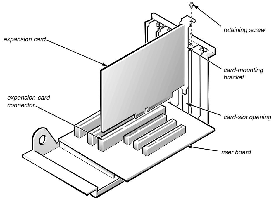
**Figure 5-15. Expansion-Card Removal**
