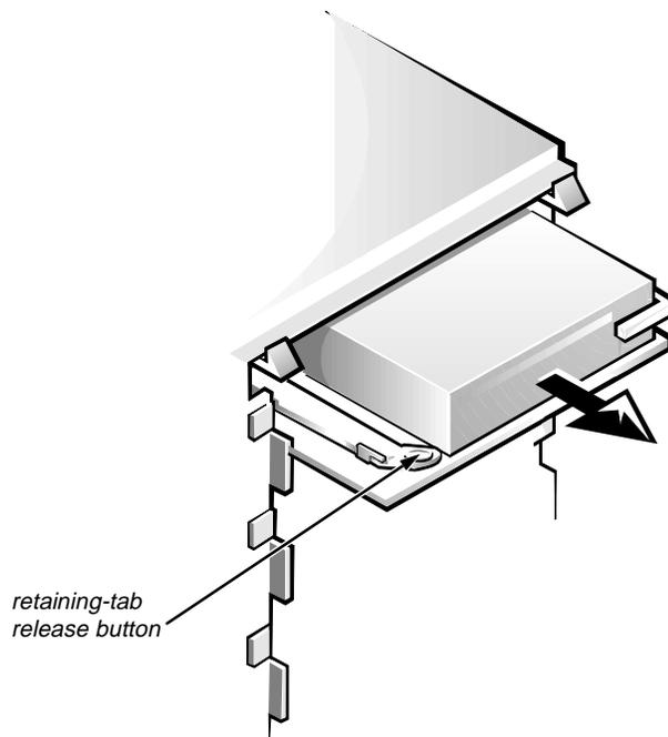
**Figure 6-8. 3.5-Inch Drive Assembly Removal**
