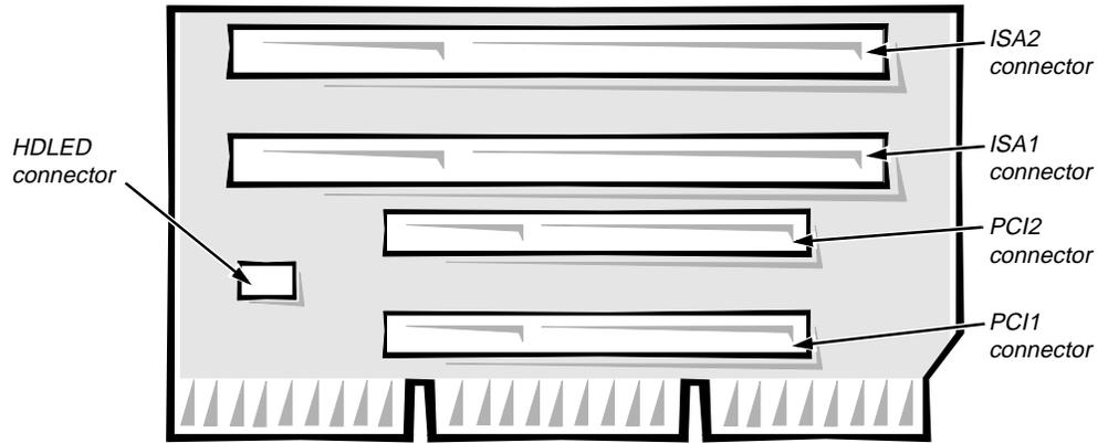
**Figure 1-6. Riser Board for the Low-Profile Computers**
