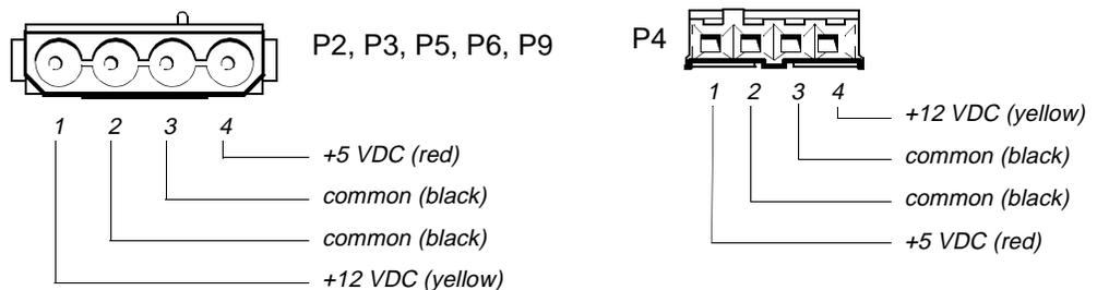
**Figure 1-12. DC Power Connectors P2 (Midsize and Mini Tower), P3, P4, P5, P6, and P9**
