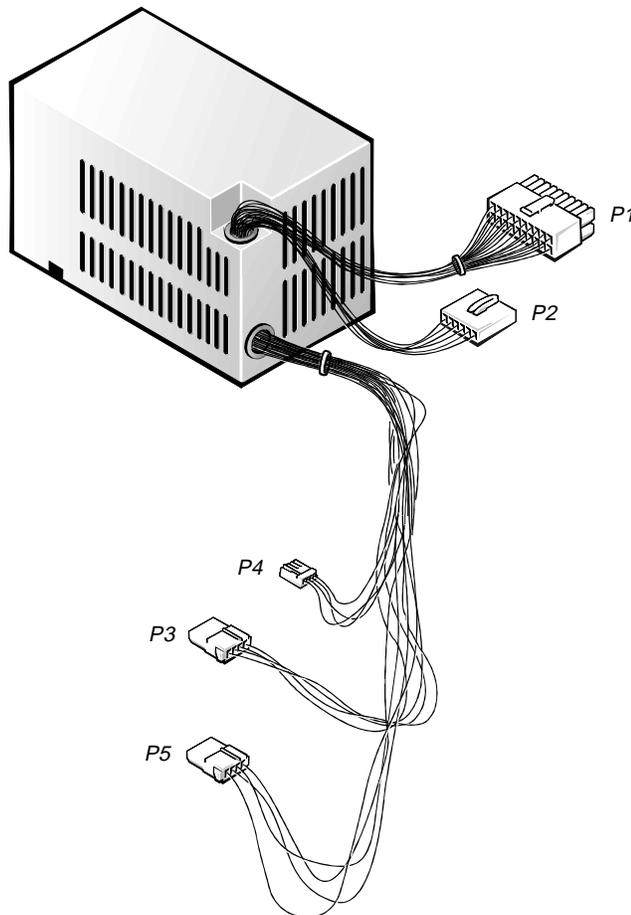
**Figure 1-14. DC Power Cables for the Low-Profile Computers**
