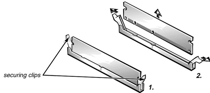
**Figure 4-14. DIMM Removal**
