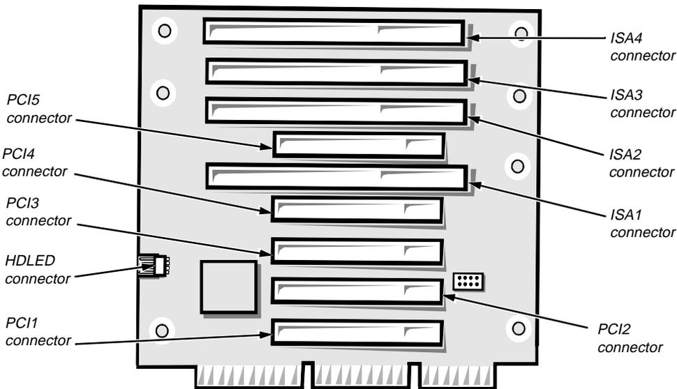
**Figure 1-9. Riser Board for the Mini Tower Computers**
