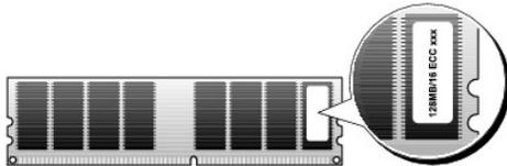
🔧 **NOTE:** Always install DDR memory modules in the order indicated on the system board.
