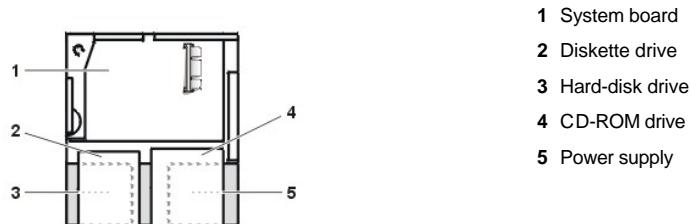
Figure 2 shows the chassis with the cover removed.
