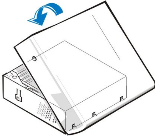
4. If your computer has a mini tower chassis, replace the computer cover as follows:
