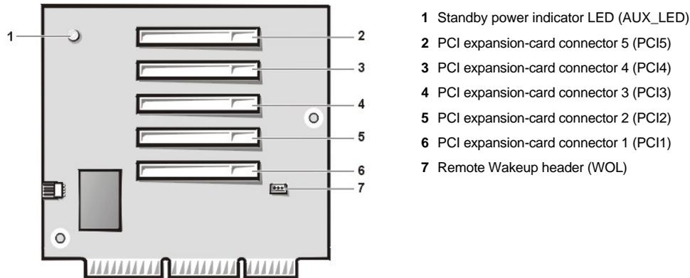
**Figure 8. Mini Tower Chassis PCI/ISA Riser Board**
