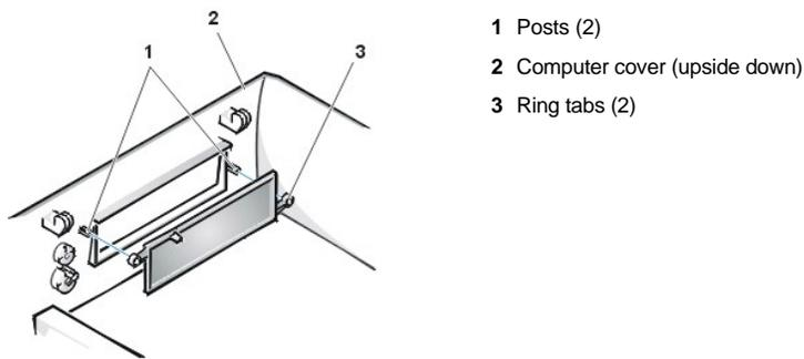
To replace the front-panel insert for the 5.25-inch bay, work from inside the cover. Position the insert behind the bay opening, insert the two ring-tabs (see [Figure 1](#)) over the posts on the inside of the opening, and firmly press both ends of the insert into place.
