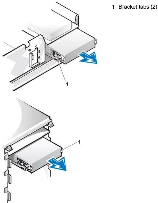
If a drive is already installed in the bay and you are replacing it, disconnect the DC power cable and interface cable from the back of the drive before you slide the bracket out of the bay.
