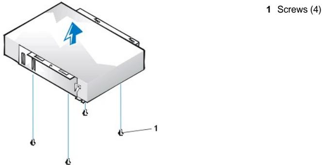
5. Attach the bracket to the new drive.
