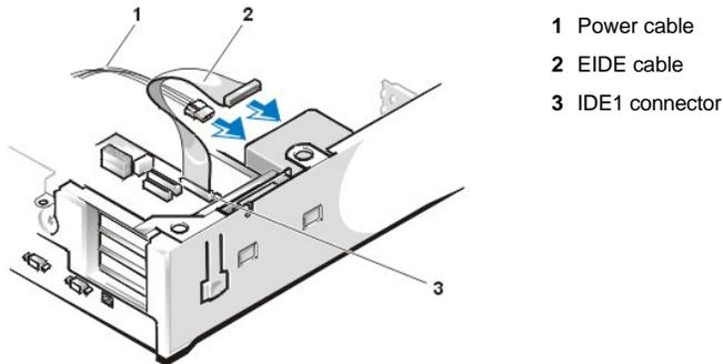
10. If it is not already connected, connect the other end of the EIDE cable to the IDE1 connector on the system board.
