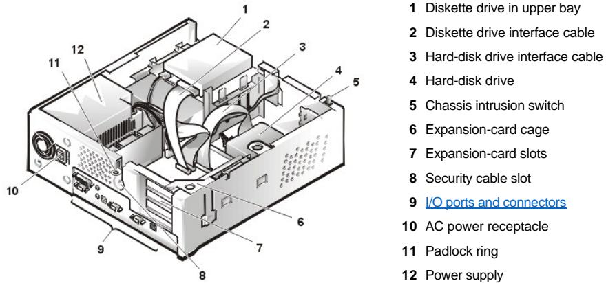
**Figure 7. Inside the Midsize Chassis**
