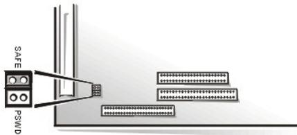
Jumpers are small blocks on a circuit board with two or more pins emerging from them. Plastic plugs containing a wire fit down over the pins. The wire connects the pins and creates a circuit.
