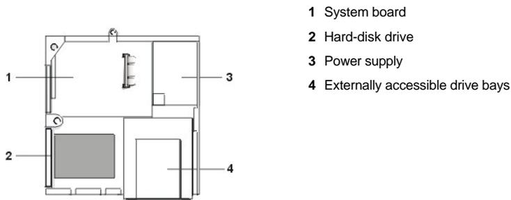
**Figure 3. Midsized Chassis Orientation View**
