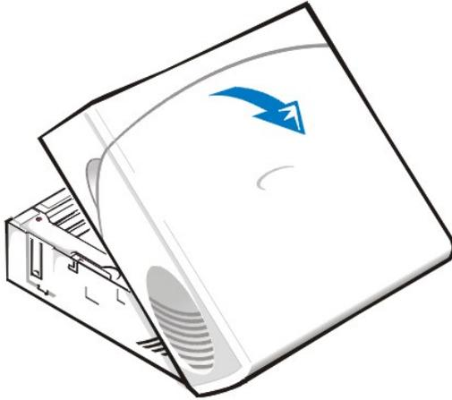
**Figure 2. Removing the Low-Profile or Midsize Computer Cover**
