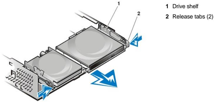
5. Remove the drive bracket from the chassis.
