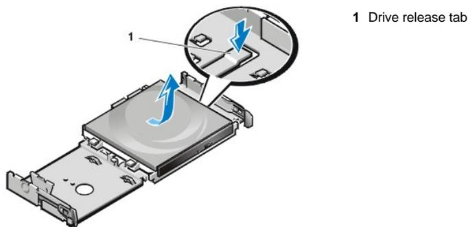
4. Install the new drive in the chassis.
