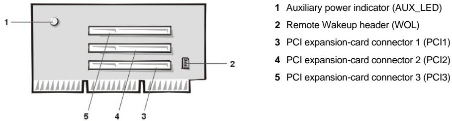
**Figure 4. Low-Profile Chassis PCI/ISA Riser Board**
