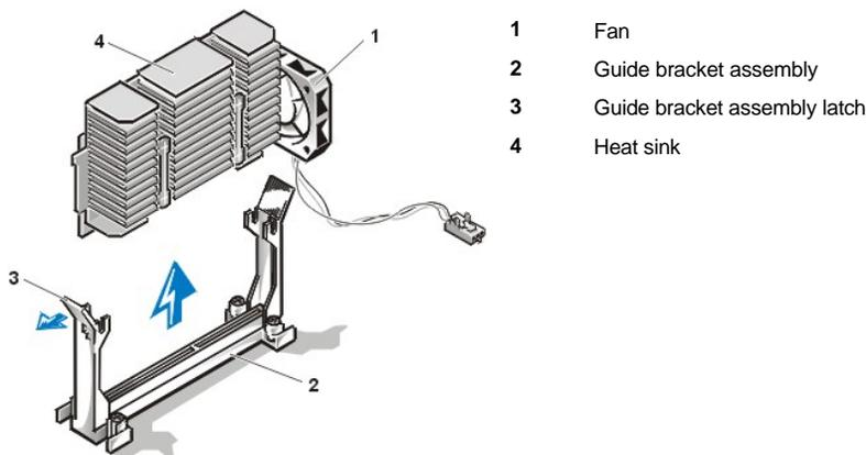
5. Reconnect the fan cable (if necessary).
