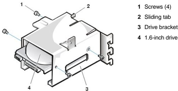
7. Reinstall the hard-disk drive bracket in the chassis (see Figure 14).
