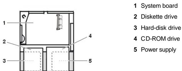
**Figure 2. Low-Profile Chassis Orientation View**
