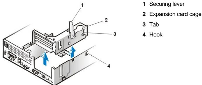
4. Slide the expansion-card cage out of the chassis.
