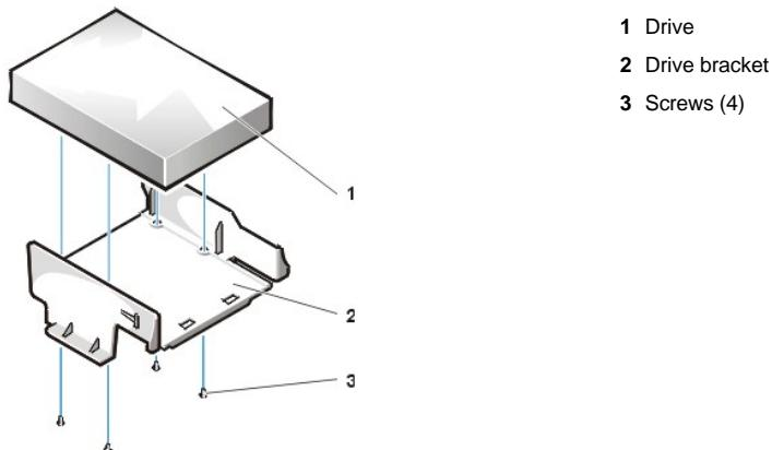
**Figure 12. Hard-Disk Drive/Bracket Replacement**
