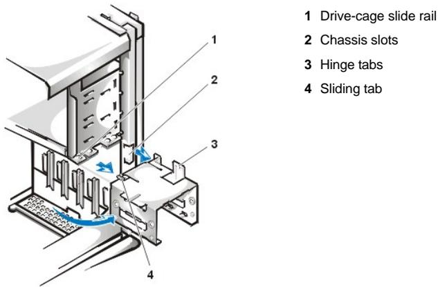
5. Slide the drive into the chosen bay of the bracket, orienting the drive so that the connectors on the back of the drive will face the back of the chassis when you reinstall the bracket (see Figure 13).
