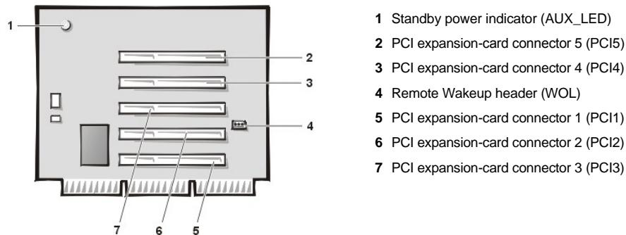
**Figure 6. Midsize Chassis PCI/ISA Riser Board**
