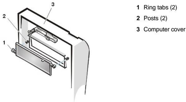
To replace a front-panel insert for a 5.25-inch bay, work from inside the bezel. Insert the two ring-tabs (one on each end of the insert) over the posts on the inside of the bay opening, and firmly press both ends of the insert into place (see [Figure 3](#)).
