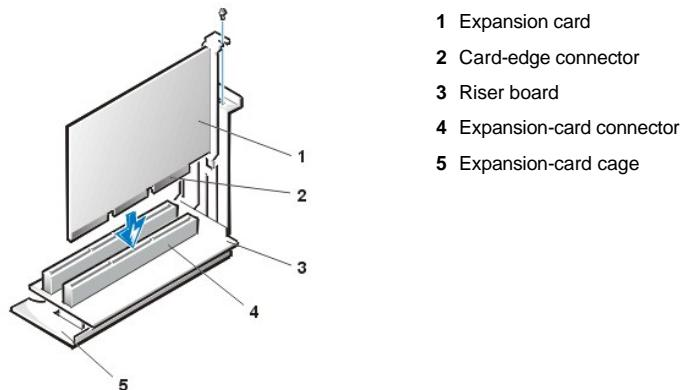
**Figure 11. Installing an Expansion Card in a Low-Profile Chassis**
