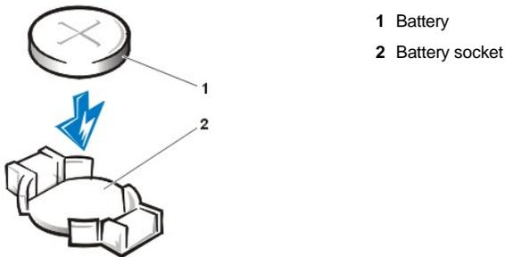
**⚠ CAUTION:** There is a danger of the new battery exploding if it is incorrectly installed. Replace the battery only with the same or equivalent type recommended by the manufacturer. Discard used batteries according to the manufacturer's instructions.
