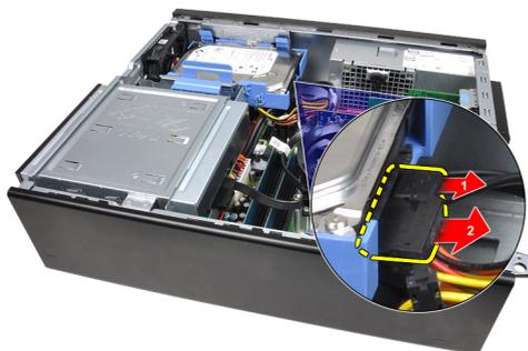
4. Press the hard-drive bracket latch towards the hard drive and lift it upward.
