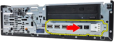
7. Remove the Input/Output panel.
