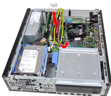
5. Lift the PCIe x1 expansion card (if any) up and out of its connector and remove it from the computer.
