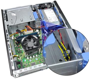
7. Pry the thermal sensor away from the chassis front and remove.
