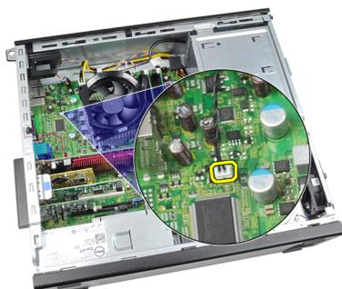
4. Unthread the thermal-sensor cable from the chassis clip.
