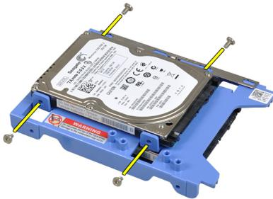
7. Flex the hard-drive bracket and then remove the two 2.5 inch hard drives from the bracket.
