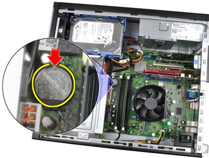
4. Lift the coin-cell battery out of the computer.
