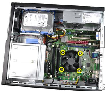
5. Lift the heat sink assembly upwards, and remove it from the computer. Lay the assembly with the fan facing downwards, and with the thermal grease facing upwards.
