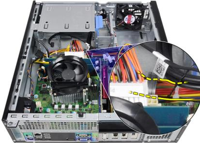
8. Remove the screws that secure the power supply to the back of the computer.
