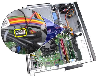
4. Unthread the speaker cable from the chassis clip.
