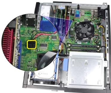
4. Slide the intrusion switch toward the chassis bottom and remove it from the system board.
