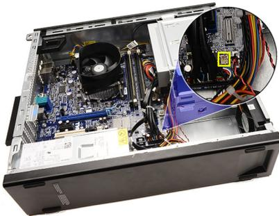
5. Unthread the thermal-sensor cable from the chassis clips.
