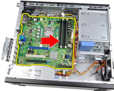
11. Remove the system board from the chassis.
