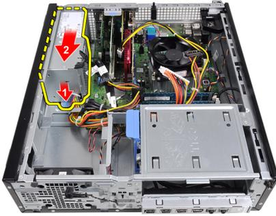
10. Lift the power supply out of the computer.
