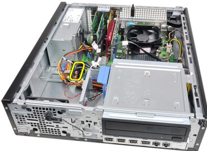
5. Remove the screw that secures the Input/Output panel to the chassis.
