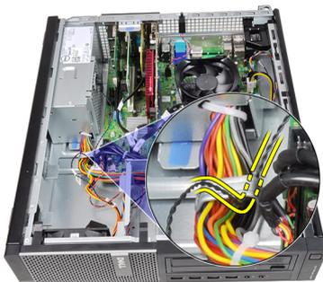
5. Pry the thermal sensor away from the power supply and remove from the chassis.
