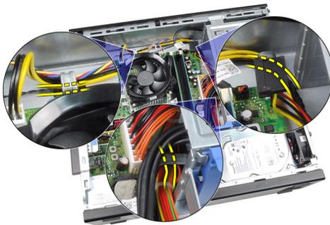
6. Unthread the thermal-sensor cable from the chassis clip.
