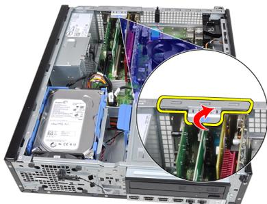
4. Pull the release lever away from the PCIe x16 card to release the securing tab from the dent in the card. Then, ease the card up and out of its connector and remove it from the computer.
