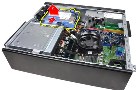
5. Flex the hard-drive bracket and then remove the single 3.5 inch hard drive or two 2.5 inch hard drives from the bracket.
