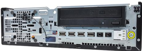
6. Slide the Input/Output panel towards the right of the system to release from chassis.
