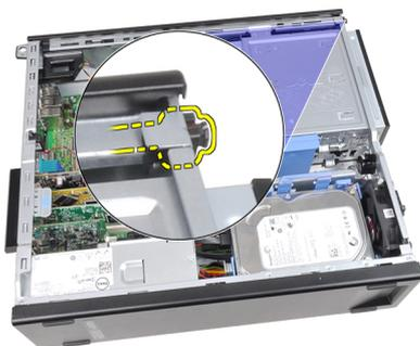
6. Slide the power-switch cable out through the front of the computer.
