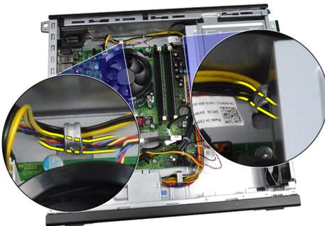
6. Slide the four grommets inward and through the slots in the front of the computer.
