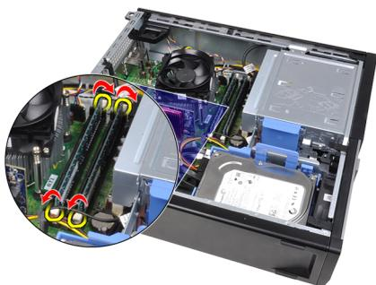
4. Lift the memory modules out of the connectors on the system board.
