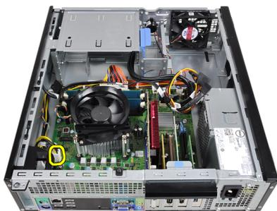
5. Unthread the 4-pin power cable from the chassis clips.
