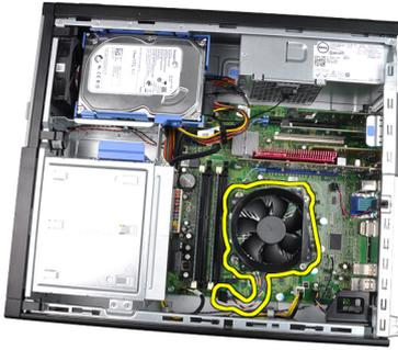
6. Press the release lever down and then move it outward to release it from the retention hook that secures it.
