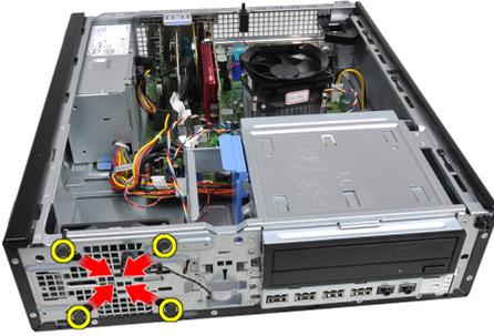
7. Lift and remove the system fan out of the computer.
