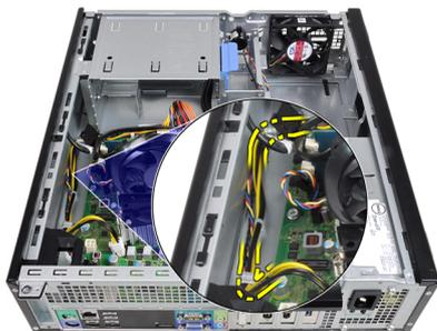
6. Disconnect the 24-pin power cable from the system board.
