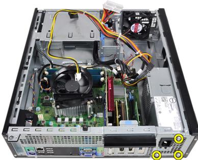
9. Push in on the blue release tab beside the power supply, and slide the power towards the front of the computer.
