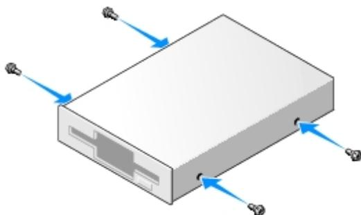
3. Align the shoulder screws on the floppy drive with the shoulder screw slots, and gently slide the drive into the bay until it clicks into place.
