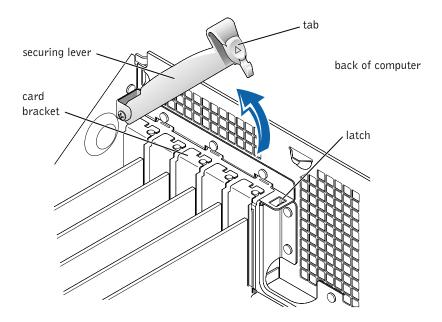
7 To remove the card, grasp the card by the top corners and lift it out. If the card is difficult to remove, gently ease the card back and forth to remove it from the connector.
