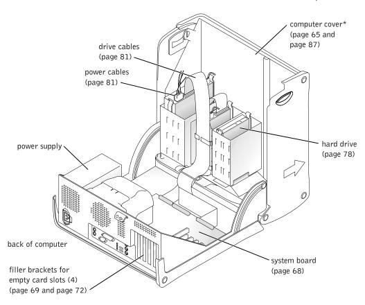
Depending on the types of drives installed in your computer, the cover may not open as widely as shown in the figure.
