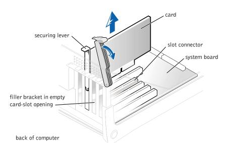
**HINT:** The AGP card is removed from the following illustration to provide a better view of the inside of your computer.
