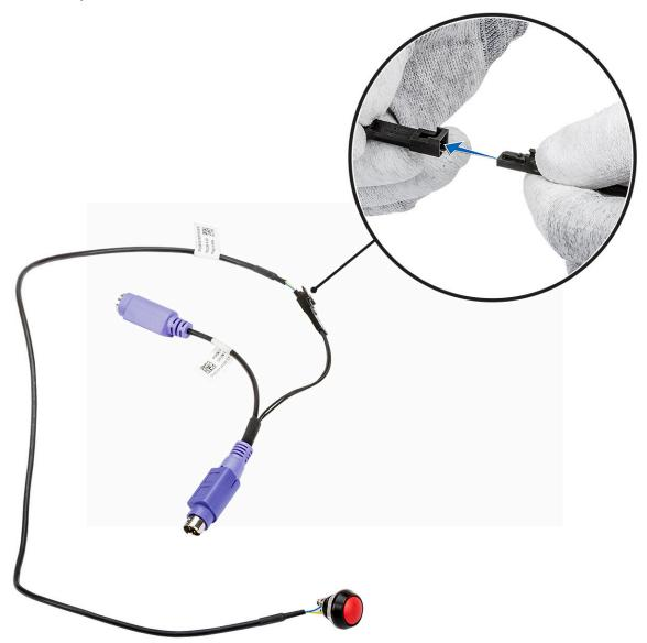
3. Pull the sleeve [1] and insert the cable to the PS/2 connector on the computer [2].
