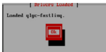
Figure 10-5. Driver Installed Successfully
