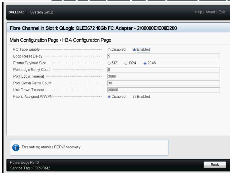
Figure 3-16. Dell System Setup: HBA Configuration
