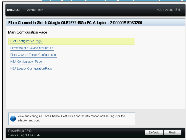
Figure 3-12. Dell System Setup: Main Configuration
