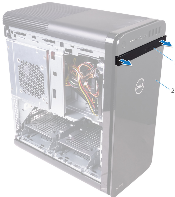
Figure 3. Removing the optical drive bezel
