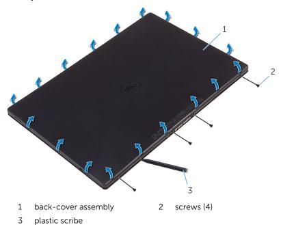
4 Carefully, lift the back-cover assembly and turn it over.
