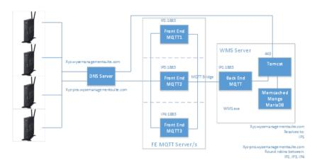
Figure 4. FE MQTT servers separate from Wyse Management Suite server
