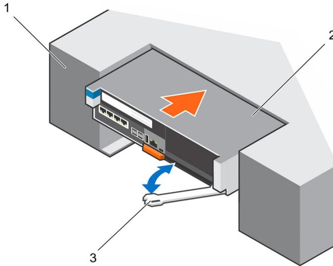
**Figure 13. Removing and Installing a Storage Controller**
