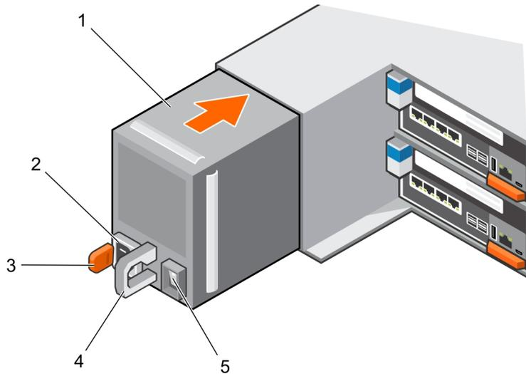
**Figure 11. Removing a Power Supply/Cooling Fan Module**
