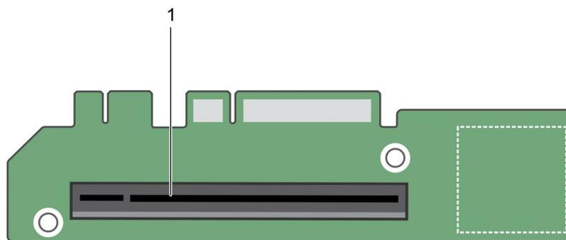
**Figure 19. I/O Card Connector Location on Riser 1**
