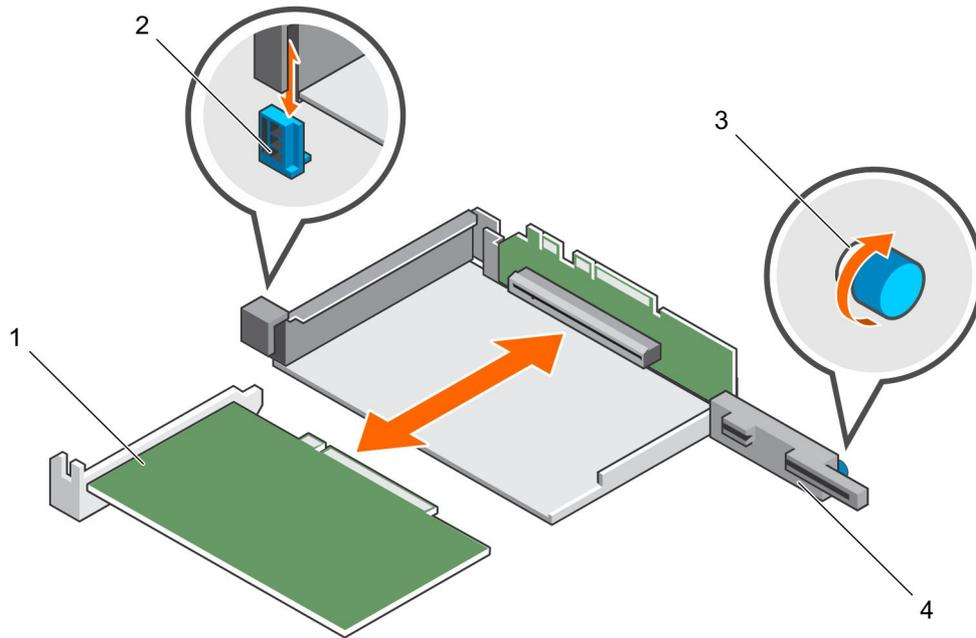
**Figure 20. Installing an I/O Card in Riser 1**
