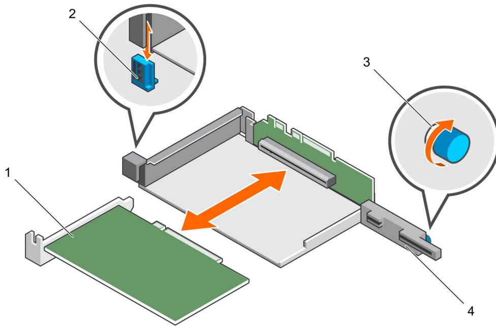
**Figure 18. Removing I/O Card From Riser 1**
