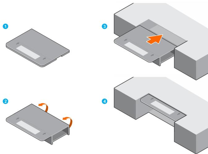
Figure 12. Installing the Service Baffle
