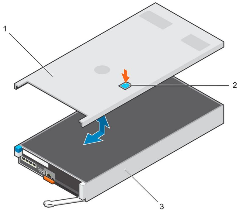
**Figure 14. Remove and Install Storage Controller Cover**
