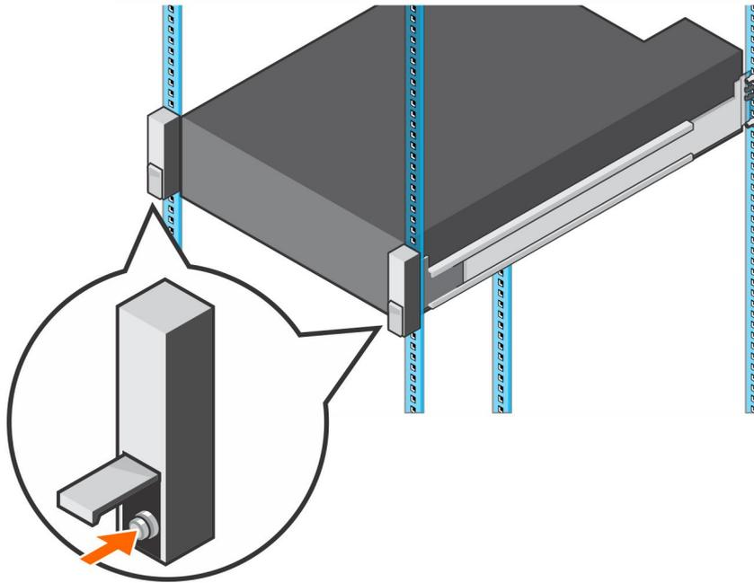
**Figure 23. Loosen the Screws**
