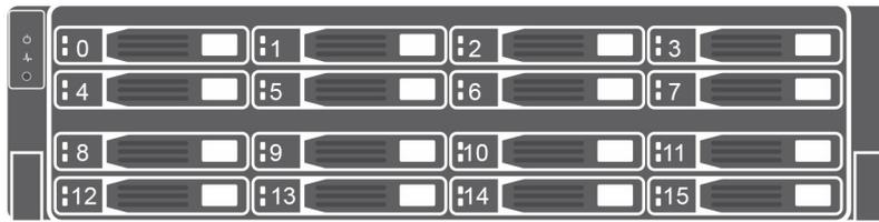
Figure 4. SCv3000 Storage System Drive Numbering
