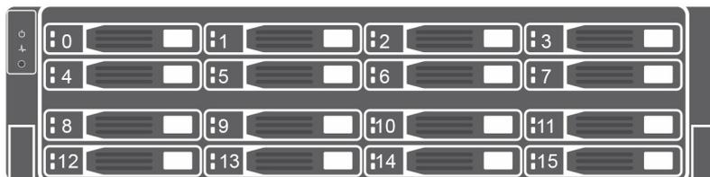
**Figure 8. SCv3000 Storage System Drive Numbering**
