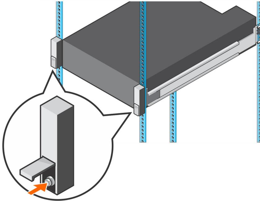
Figure 24. Tighten the Screws
