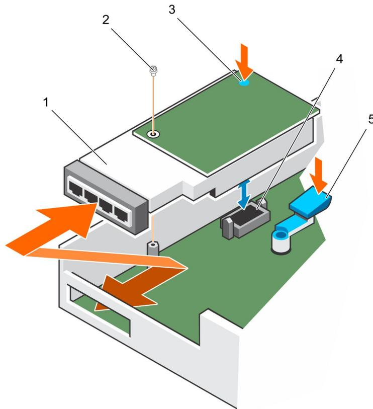
**Figure 22. Install the Mezzanine Card**
