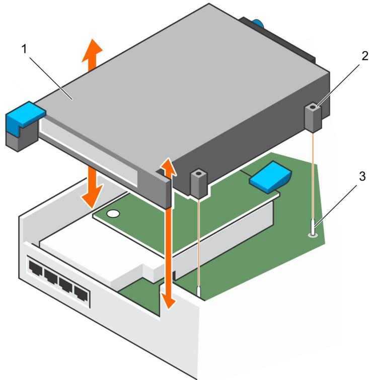
**Figure 17. Removing Riser 1**
