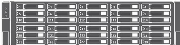
Figure 5. SCv3020 Storage System Drive Numbering
