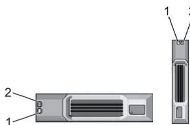
**Figure 3. SCv300 and SCv320 Expansion Enclosure Drive Indicators**
