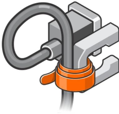
**Figure 10. Removing the Hook and Loop Strap from the Power Cable**
