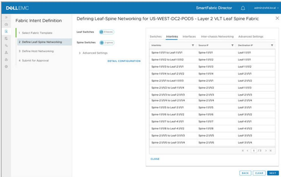
Details of interchassis configuration for Layer 2 fabric.
