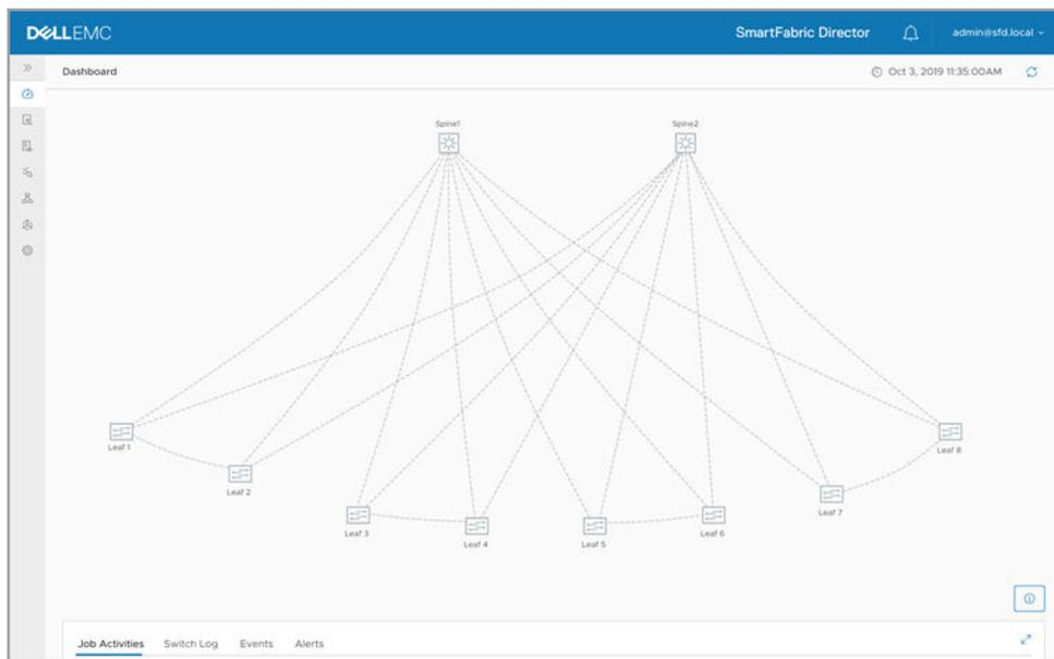
As the switches are discovered, SFD begins configuration of each switch. The progress can be viewed in the Job Activities pane at the bottom of the screen.
