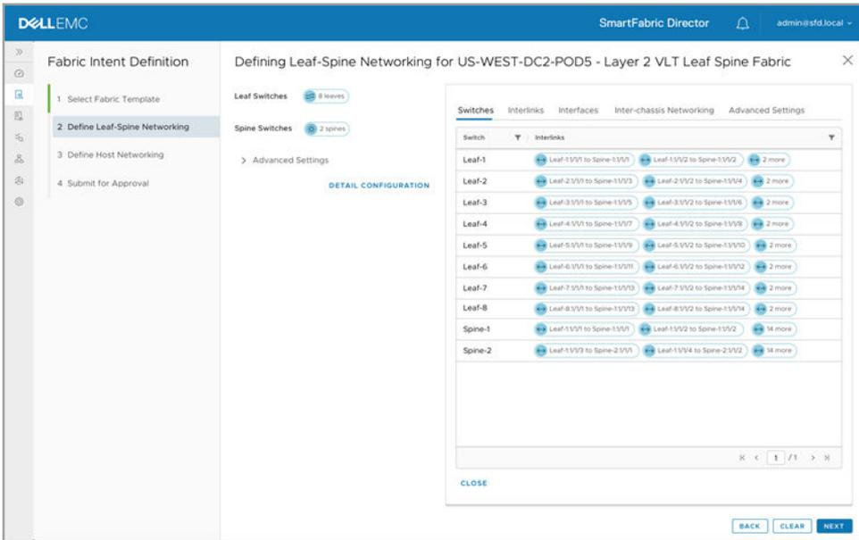
Details of interlinks configuration for Layer 2 fabric.
