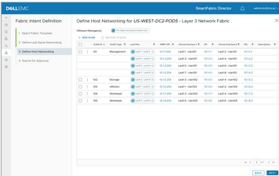
2. Associate one or more VLT pairs to a VLAN ID from the list of available VLT pairs (derived from the wiring diagram). Each leaf in the VLT pair has its own SVI IP, and each VLAN in the VLT pair has a VRRP virtual IP in the same subnet as the VLAN.
