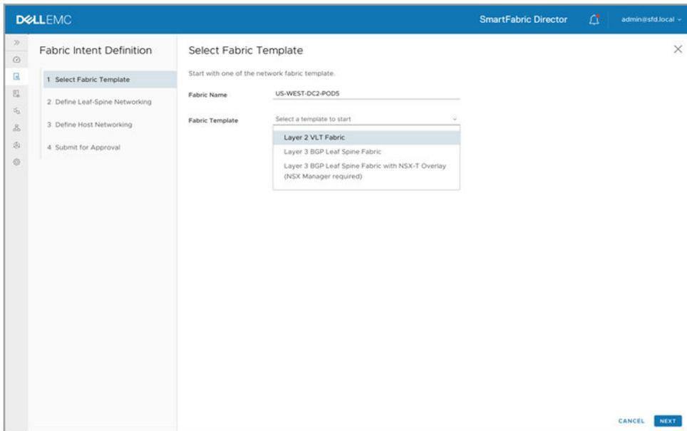
You are now ready to specify the parameters to generate configuration for the host facing ports, inter-VLAN routing, and host dual-homing. This screen also indicates the IP or DNS address of the vCenter (VMware Manager) used to manage the VMs on the hosts that are connected to this fabric.
