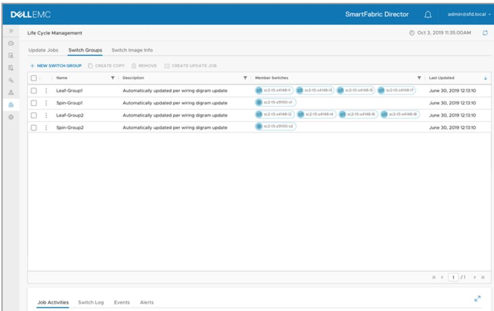
2. Enter the name for the new switch group, select the switches to add to the switch group from the active wiring diagram, enter an optional description, then click **Create**.
