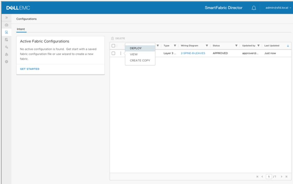
SFD starts configuring each discovered (and reachable) switch with the wanted configuration that is derived from the chosen approved Intent. SFD interfaces with each switch through the gNMI protocol for configuration, and the switches are configured simultaneously.
