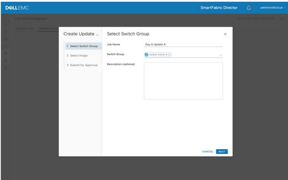
3. Specify an OS10 image including the file extension (.bin). Verify the specified image name matches the name of the image file on the remote server, then click **Next**. All switches in a switch group are updated to the specified image when the Update job is run.
