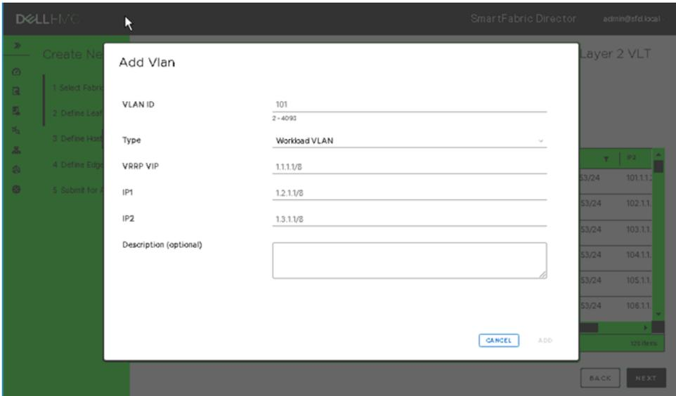
SFD creates a virtual interface on each spine, and associates it to the VLAN ID. Each virtual interface obtains an SVI IP, and each VLAN in the VLT pair obtains a VRRP virtual ip in the same subnet as the VLAN.
