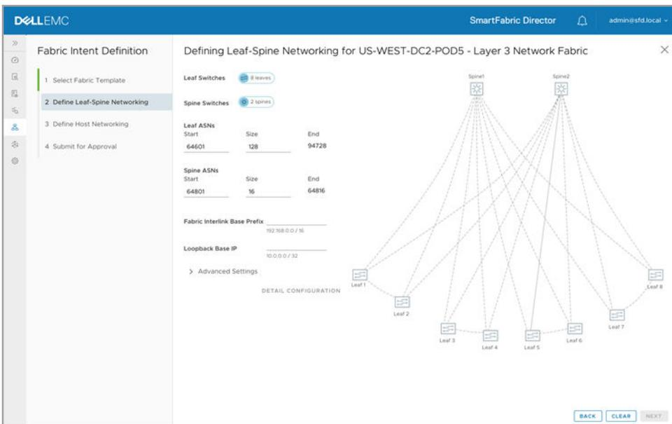
2. (Optional) Click **Detail Configuration** to view the interlinks between the leaf and spine switches, or click **Clear** to clear the specified intent, along with the detailed (per switch) configuration for the interlinks. Click **Back** to return, or click **Next** to continue.
