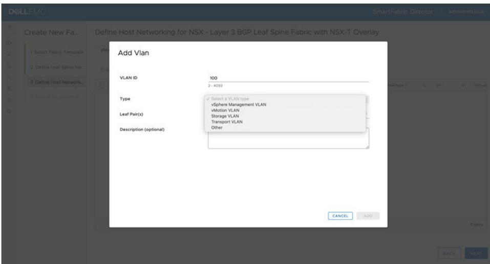
5. Assign **Leaf pair(s)** to each VLAN; repeat until you have assigned all leaf pair switches to the corresponding VLAN.
