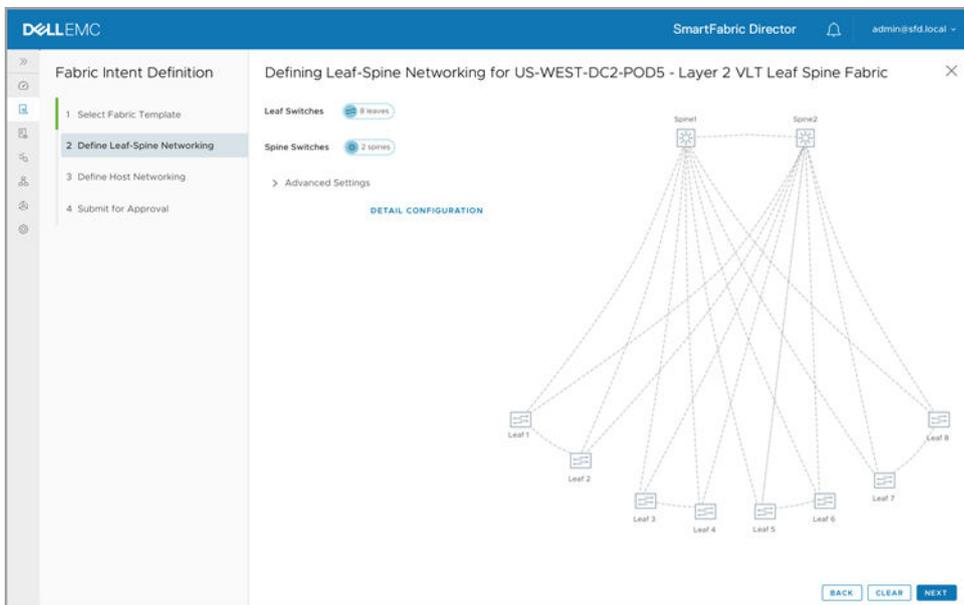
2. (Optional) Click **Detail Configuration** to view the per switch configuration, click **Clear** to clear the specified intent, along with the detailed (per switch) configuration for the interlinks. Click **Back** to return, or click **Next** to continue.
