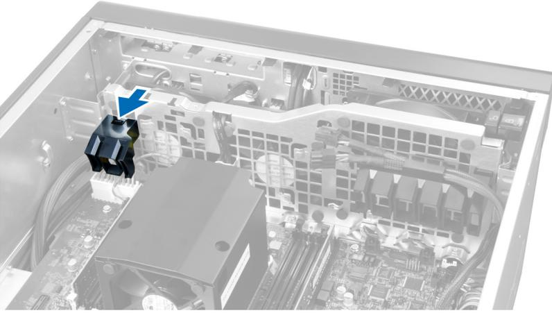
5 Lift the PCIe card retention in an upward direction to remove it from the computer.
