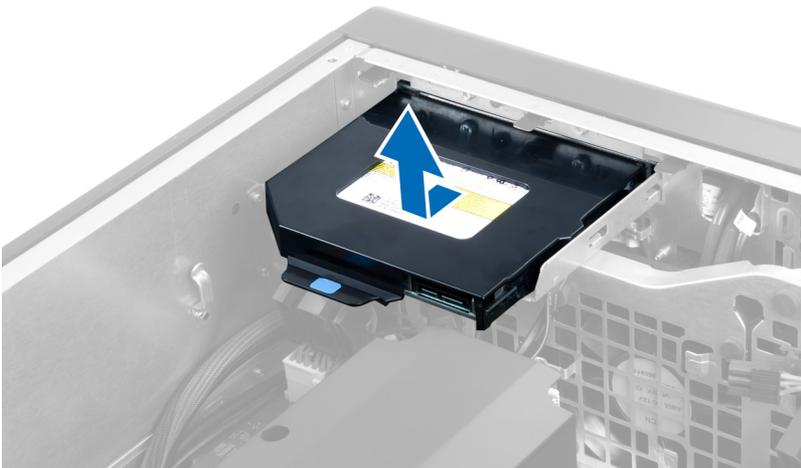
7 Flex the optical-drive bracket latches in an outward direction to loosen the optical drive from the bracket.
