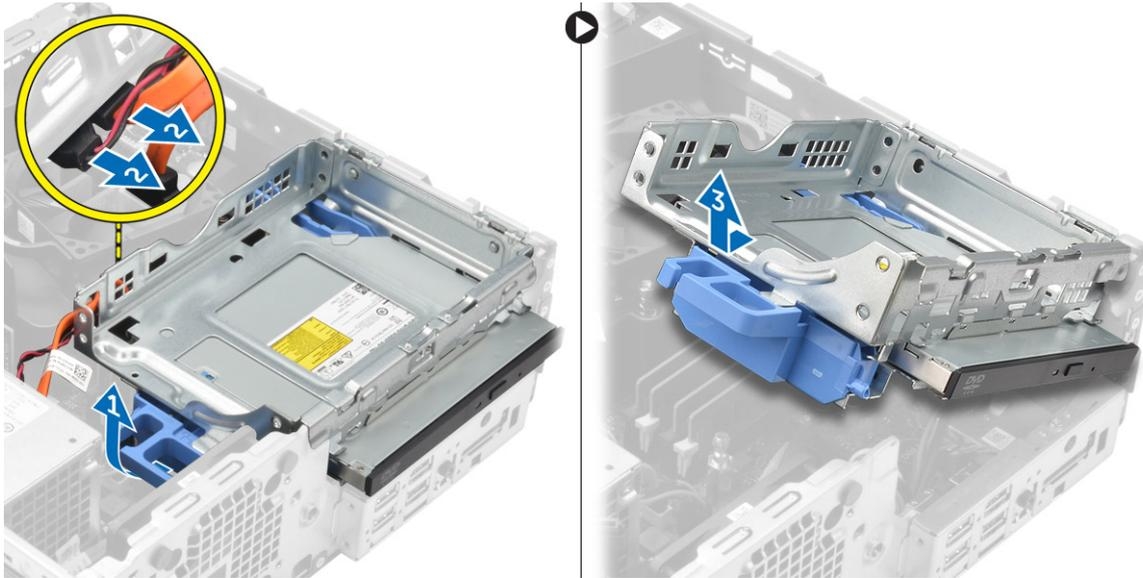
5. To remove the optical drive from the optical drive cage:
