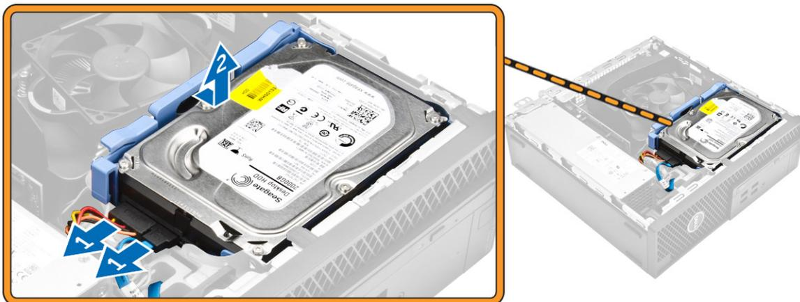
4. To remove the hard drive bracket:
