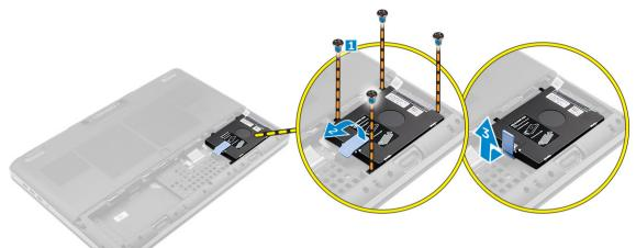
4 Remove the screws that secure the hard drive to the hard drive bracket . Lift the hard drive from the bracket .
