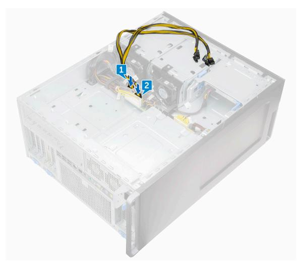
Remove the plastic clip outward [1] and route the two VGA power cables by pressing the cables [2]. Press the clip after routing the cables to lock the routed cables [3].
