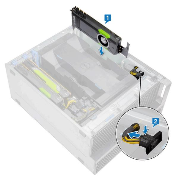
f Connect the power cable to the graphic card.
