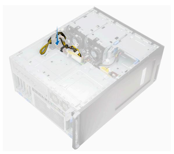
6 Connect the third VGA power cable in the slot as shown in the following image. The third cable needs to be connected in the slot which is opposite to the fan assembly.
