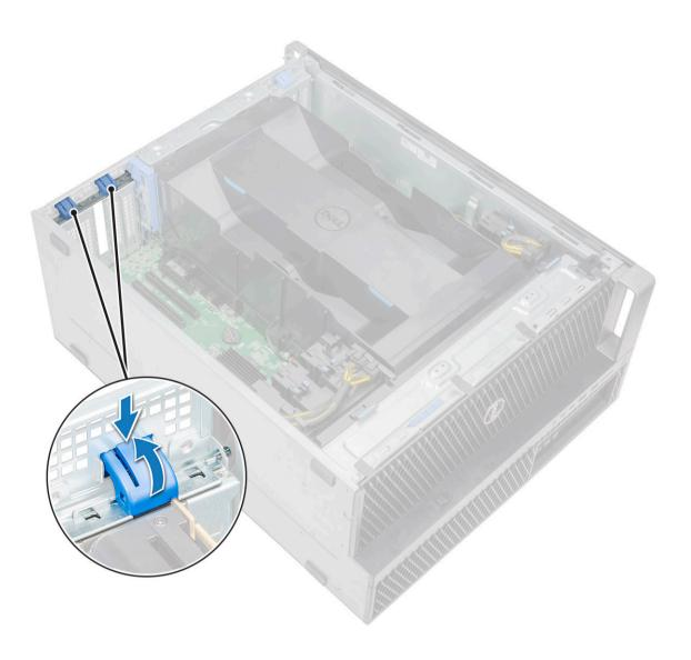
c Align and place the graphic card to the PCle slot on the system board. The following image shows the graphic card being placed on PCle slot 3. You must place the graphics card in PCle slot 2.
