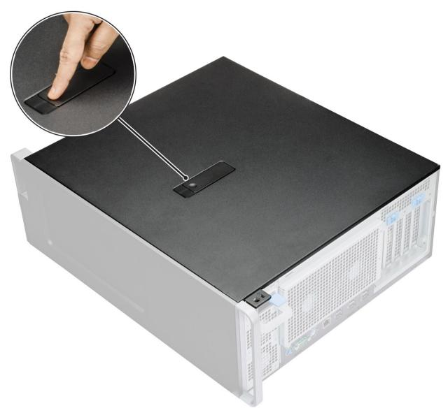
b Pull the latch [1] upward and slide the side cover outwards to remove it from the system [2].
