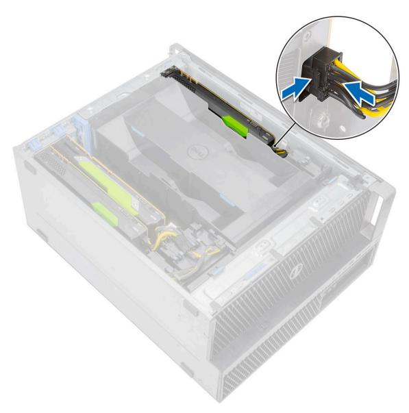
g Press and rotate the PCle latch backward to unlock the filler bracket.
