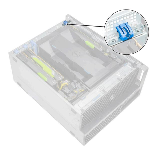
6 Align and install the side cover to the system.
