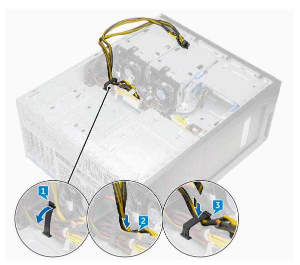
Connect the other ends of the two VGA power cables to the slots by pressing the cables.
