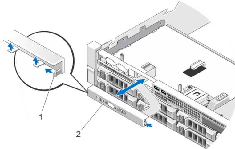
1. notches on chassis front wall (6)
