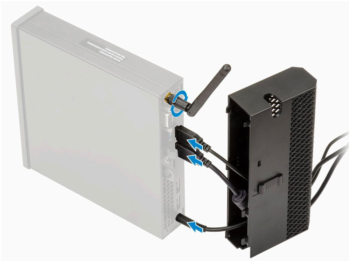
3 Align the cable cover retaining hooks into their slots on the Dell OptiPlex Micro chassis.
