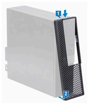
2 Gently press as shown to ensure the dust filter fits snugly onto the system.
