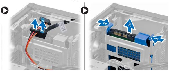
**4.** Flex the hard-drive bracket and remove the hard drive from the hard-drive bracket.
