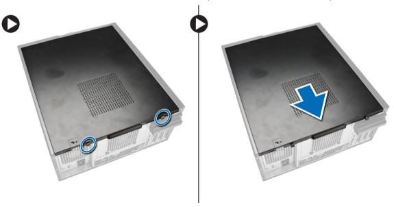
**3.** Lift the cover upward to a 45-degree angle and remove it from the computer.
