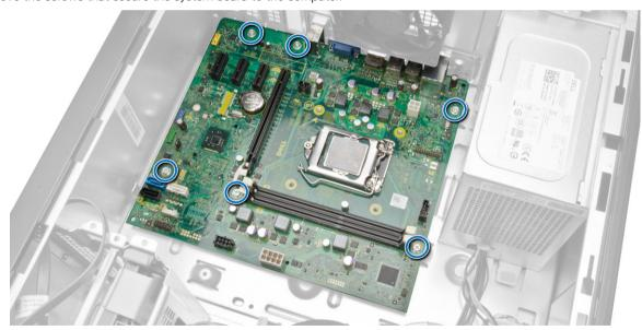
**6.** Tilt the system board at 45-degrees, and then lift the system board out of the computer.
