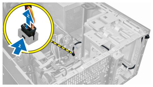
4. Release the power-switch cable from the chassis clips.
