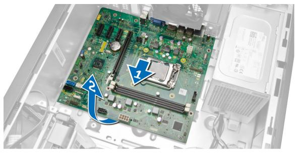
7. Lift the system board out of the computer.
