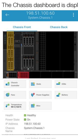
**Figure 46. Chassis dashboard (phone view)**
