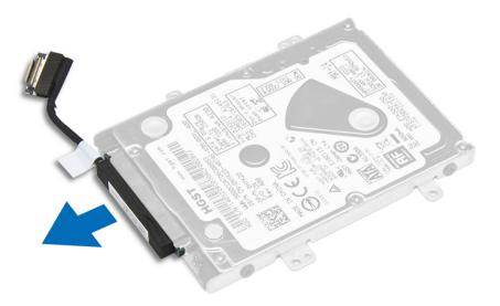
4 Remove the screws that secure the hard drive bracket to the hard drive [1] and lift the hard drive from the hard drive bracket [2].
