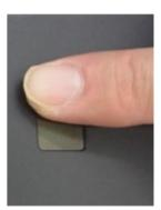
NOTE: Adjust the position of the finger to enable the reader to capture multiple scans of your fingerprint. The reader thus creates a more complete image of the fingerprint and improves the reliability of the reader.
