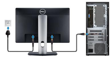
i NOTE: If your computer is shipped with an integrated graphics card only, connect the display to a display port on the back panel.
