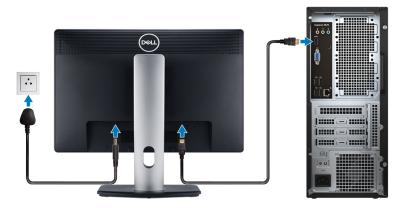
**4.** First connect the power cable to the computer and then to a power source.
