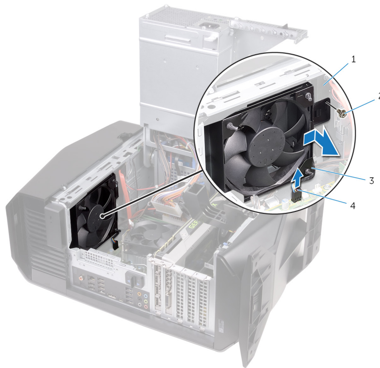
Figure 44. Removing the top-chassis fan
