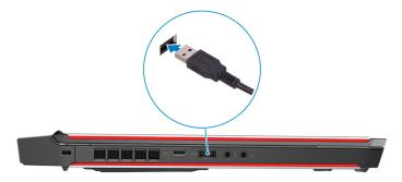
6. Connect a USB Type-C to Type-A dongle to the USB 3.1 Gen 2 (Type-C) port at the left side of your computer.
