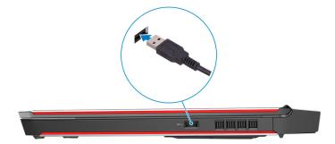
4. Connect a USB Type-C to Type-A dongle to the Thunderbolt 3 (USB Type-C) port on the back of your computer.
